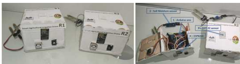
Fig. 7: Practical implementation of the developed IoT-based irrigation system including Arduino board, Wi-Fi module, electronic sensors of temperature, humidity and soil moisture.
