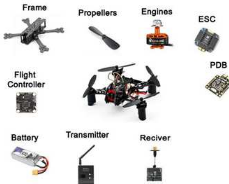
Fig. 2: Basic components of a drone
