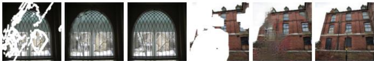
Fig. 8 - Partial convolution Results (Fawzi, et al. 2016). (a) The masked image on the left; (b) The recovered image in the middle; (c) The real image on the right.
