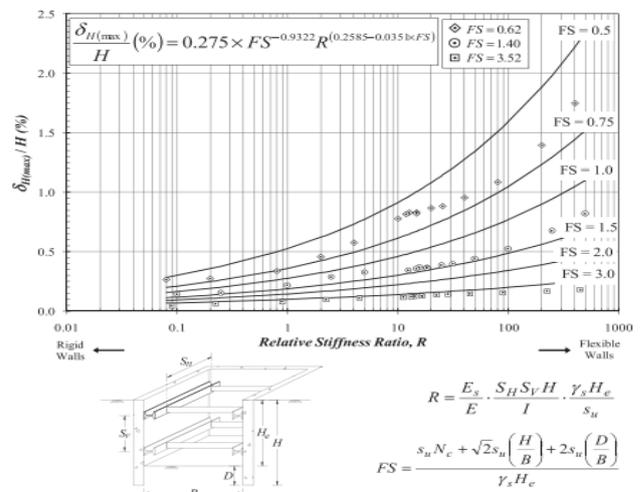
Fig. 2 Zapata 2012 Design Chart
