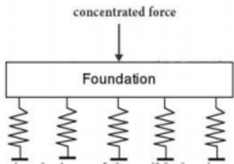
Fig. 12 The concept of modulus of subgrade reaction
