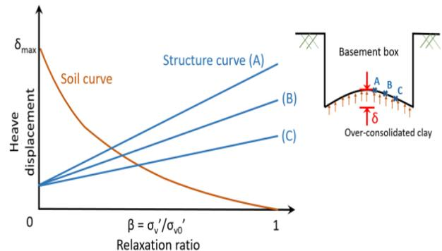
Fig. 6 Schematic Diagram Showed Relaxation ratio methods
