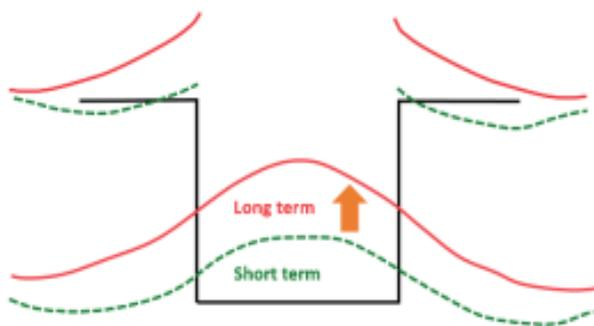
Fig. 5 Schematic Diagram Showed heaves associated soft soil
