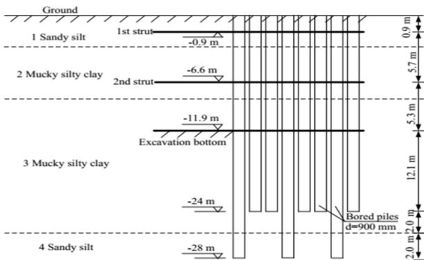
Fig. 9 Layout of Case study and comparison between calculated and measured heave. Changjie XU (2013)
