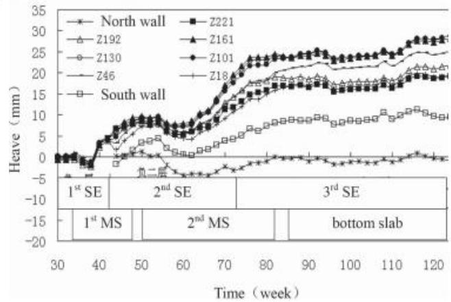
Fig. 8 Measured Heave in Case Study used in G. Zheng Study (2012)
