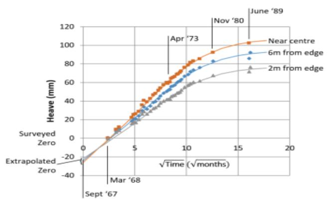
Fig. 10 Measured heave of underground vault in British library
