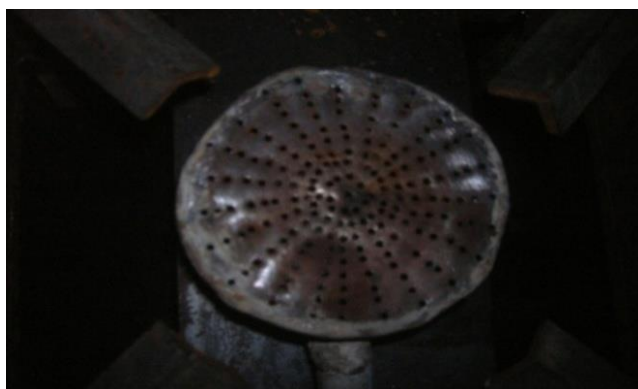
Figure 5: Burner ports design of prototype burner
