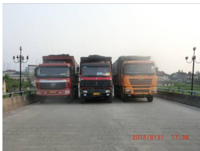
Fig. 21. Eccentric truck loads in the field.
