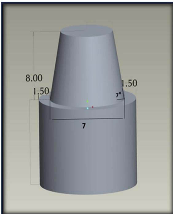
Fig. 1. Diagrammatic drawing for Stainless steel die.
