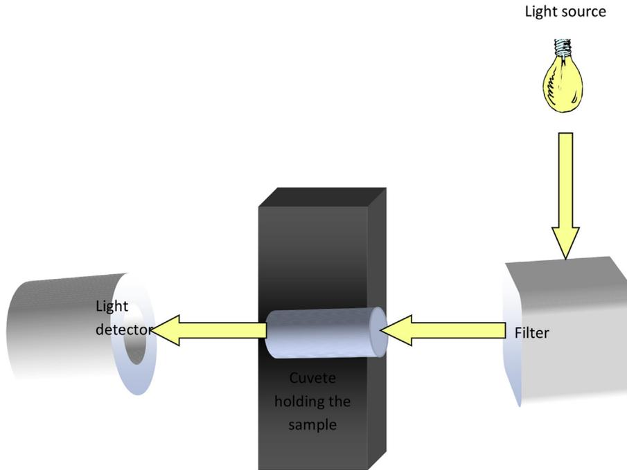
Fig. 3. Diagrammatic drawing for Unicam Helios Spectrophotometer.
