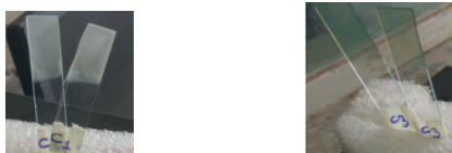
Fig. 2: Photo image of zinc sulfide thin film and copper zinc sulfide thin films on the substrate.
