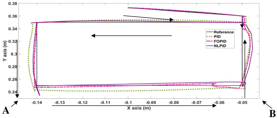
Fig. 20 - the trajectory planning of PIDs family control technics.
