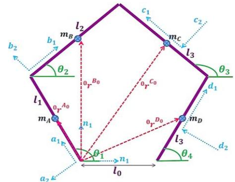
**Fig. 4 - Dynamics of the Pantograph**
