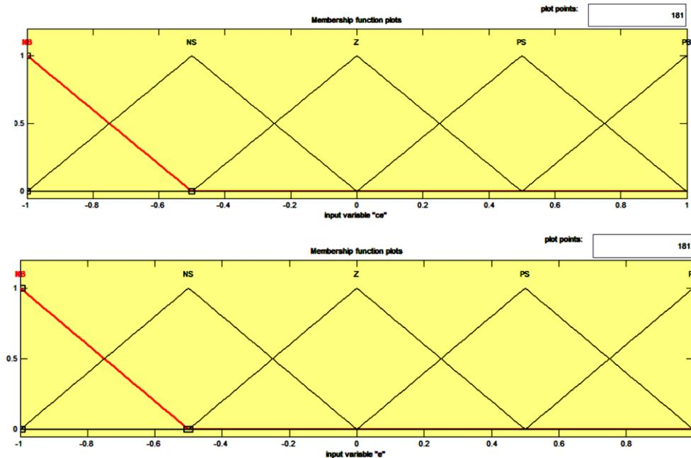
Fig. 13 - the input membership for fuzzy PD+I control.
