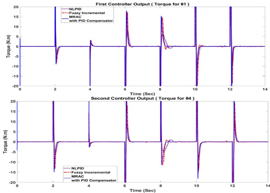
Fig. 24 -The controller output (torque N.m) is shown for the first and second controller respectively for NLPID ,Fuzzy PD+I, and MRAC with PID Compensator.
