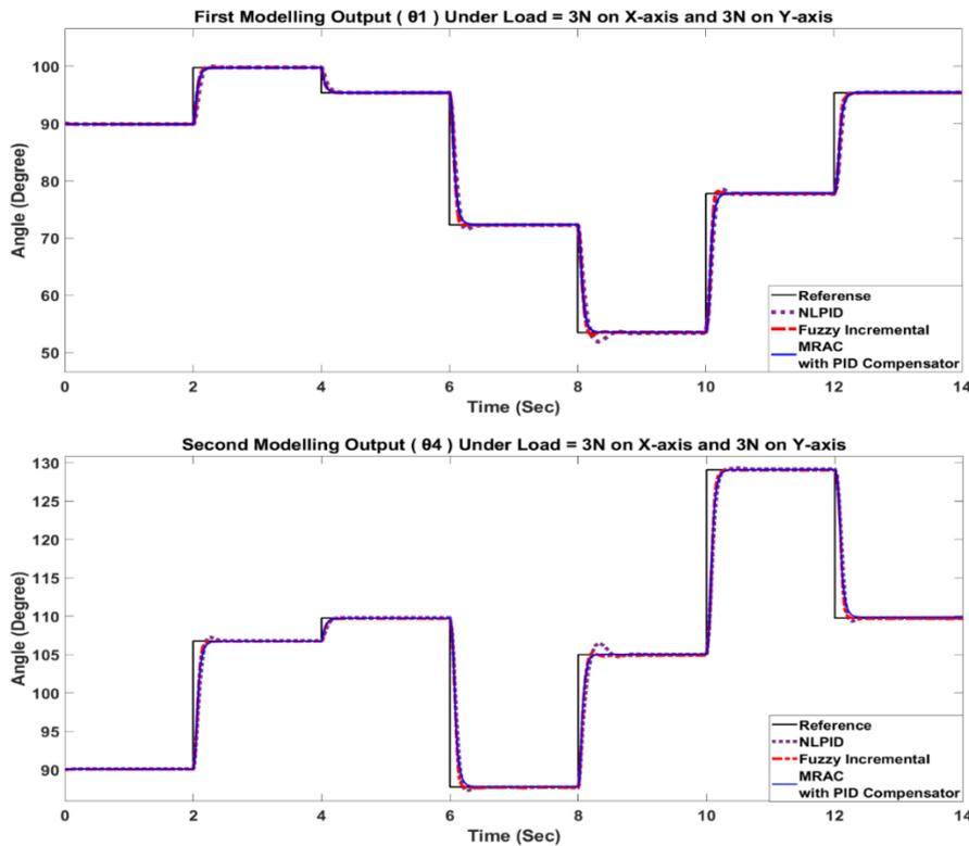
**Fig. 27 - Position response of  $\theta_1$  &  $\theta_4$  under load, through NLPID, Fuzzy PD+I, and MRAC.**
