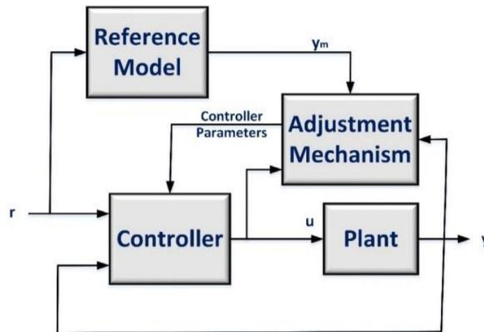
Fig. 8 - A Block diagram of a general MRAC controller [64].
