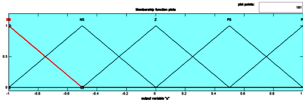
Fig. 14 - The output membership for fuzzy PD+I control.
