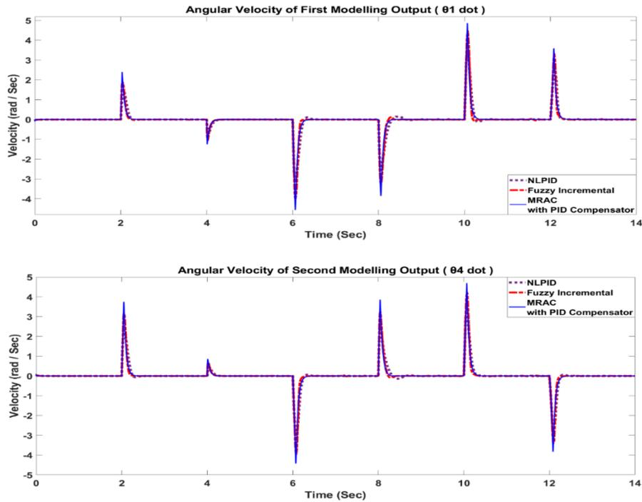
Fig. 23 - The position response of  $\theta_1$  and  $\theta_4$  through NLPID, Fuzzy PD+I, and MRAC, Control.
