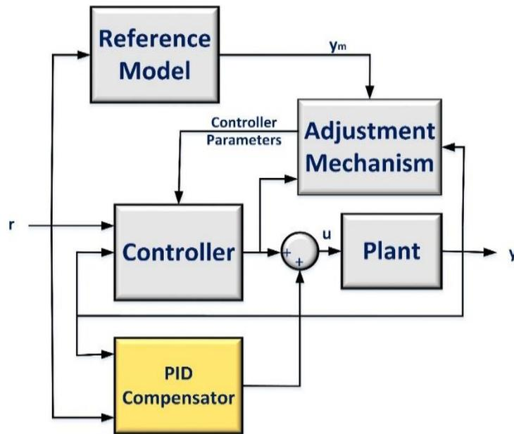
Fig. 10 - Block illustration of MRAC with PID compensator.
