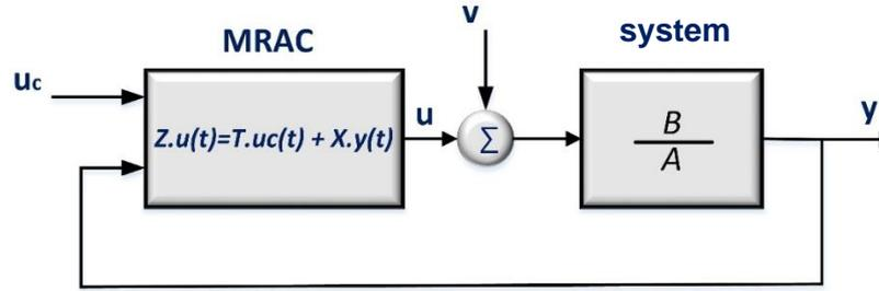
Fig. 9 - A overall linear controller with two marks of freedom.
