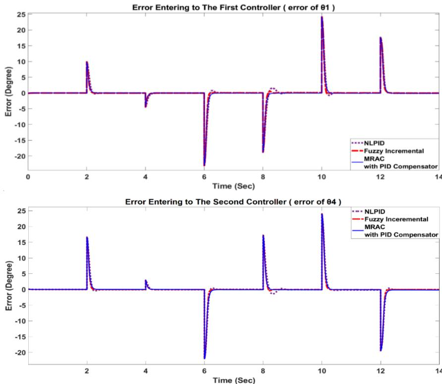
Fig. 26 - The entering error to the controller is shown for the first controller and the second one respectively.
