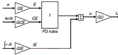
Fig. 12 - Structure of Fuzzy PD+I controller.
