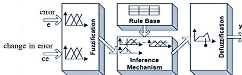
Fig. 11 - Fuzzy logic control construction [57].
