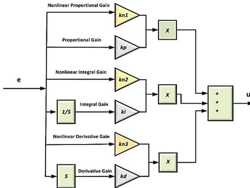
Fig. 7 - The enhanced Nonlinear PID Controller structure.
