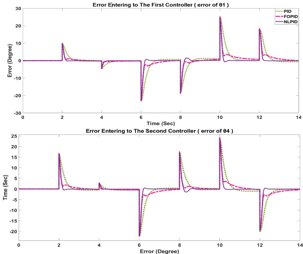
Fig. 21 -The entering error to the controller is shown for the first controller and the second one respectively.
