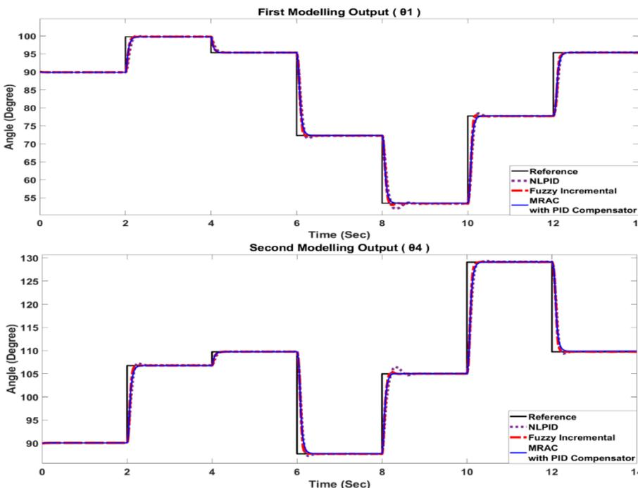
**Fig. 22 - The position response of  $\theta_1$  &  $\theta_4$  through NLPID, Fuzzy PD+I, & MRAC techniques.**
