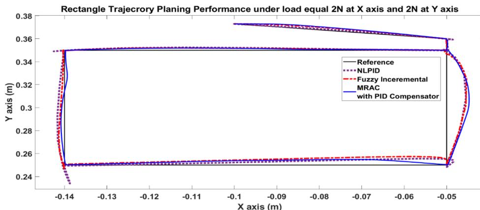
Fig. 28 -- The trajectory planning of NLPID, Fuzzy PD+I, and MRAC with PID compensator control technics.
