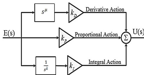
**Fig. 6 - FOPID block diagram.**
