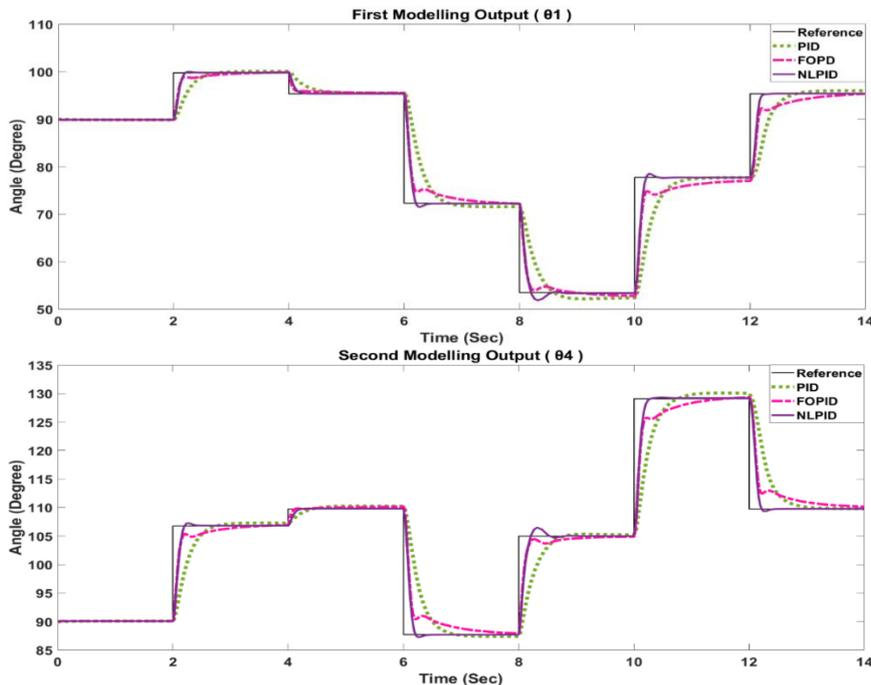
Fig. 17 - The position response of  $\theta_1$  and  $\theta_4$  through the PIDs Family control techniques.
