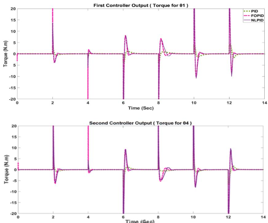
Fig. 19 - The controller output (torque N.m) is shown for the first and second controllers respectively.
