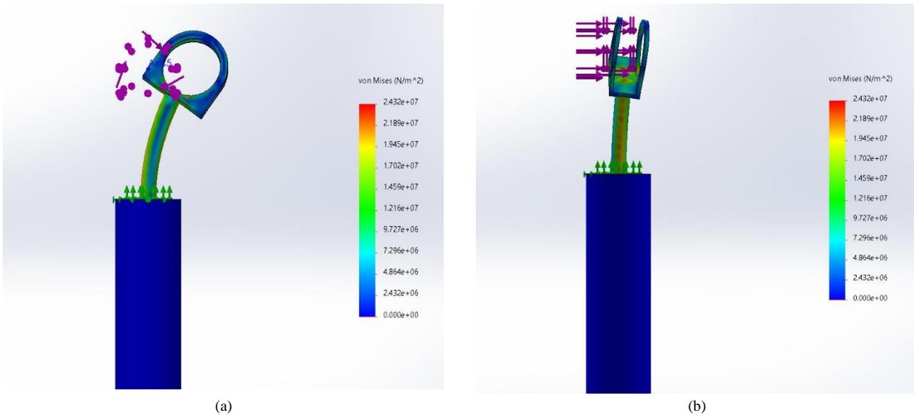
Figure 8. von Mises Stresses for the Single-Rotor Test Rig: (a) Elevation View, (b) Side View
