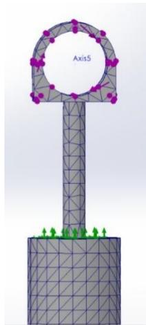
**Figure 6. Mesh of the Single-Rotor Test Rig**
