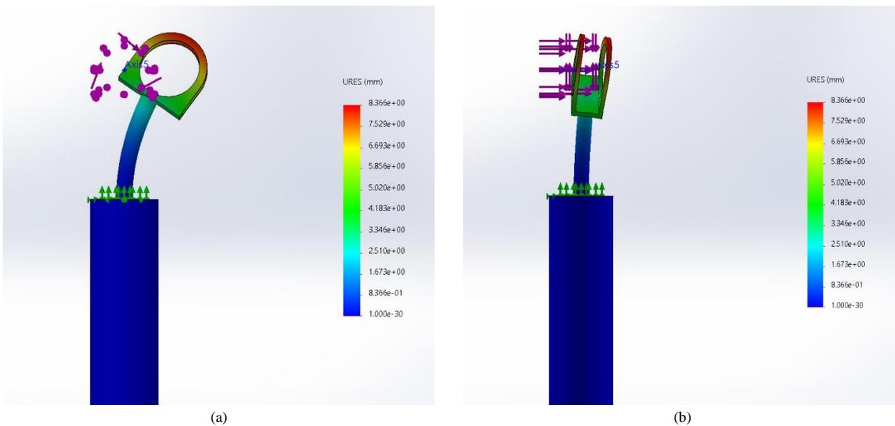
Figure 9. Deflections of the Single-Rotor Test Rig: (a) Elevation View, (b) Side View
