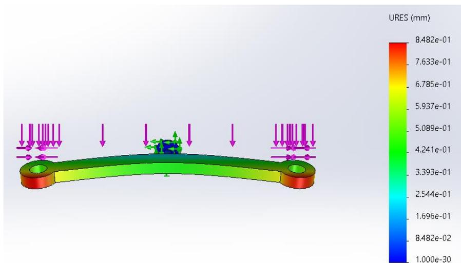
**Figure 12. Deflections of the Twin-Rotor Test Rig: Top View**
