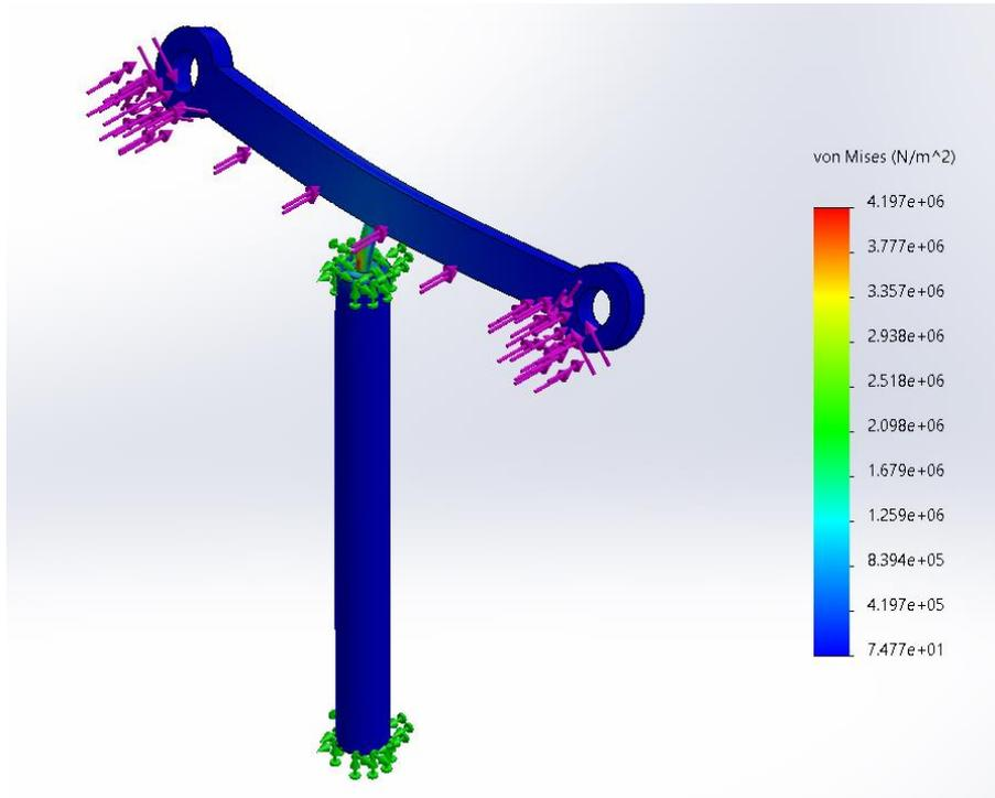
Figure 10. von Mises Stresses for Twin-Rotor Test Rig: Isometric View
