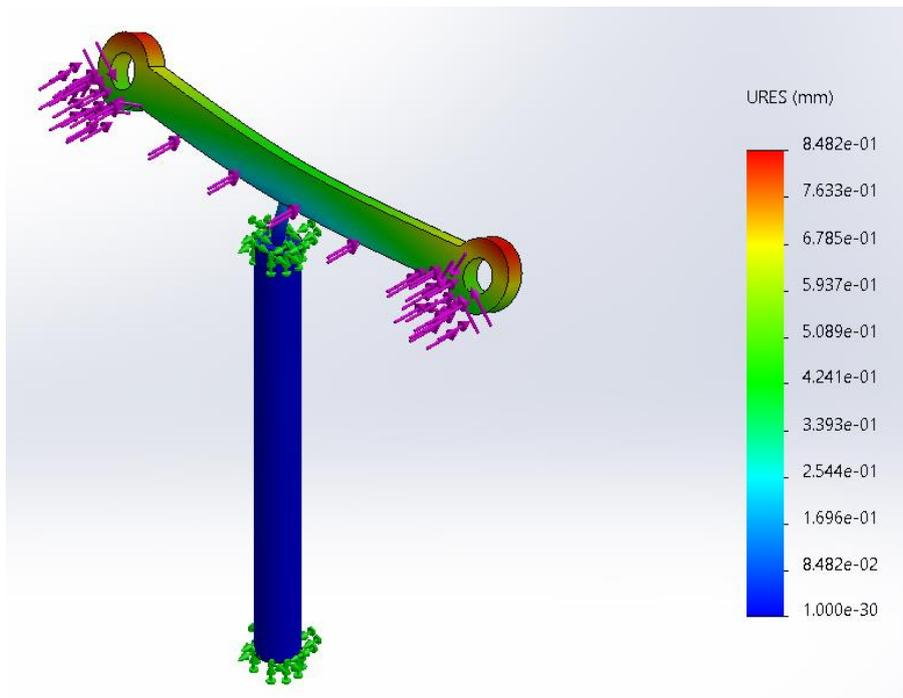
Figure 11. Deflections of the Twin-Rotor Test Rig: Isometric View
