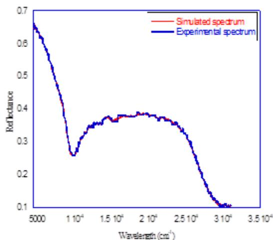
**Figure 2.** An illustration of fitting of the experimental to simulated spectra using the SCOUT software.
