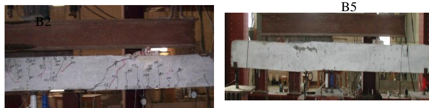
Figure 8. Flexural shear failure: Crack pattern at failure for B2 and B5
