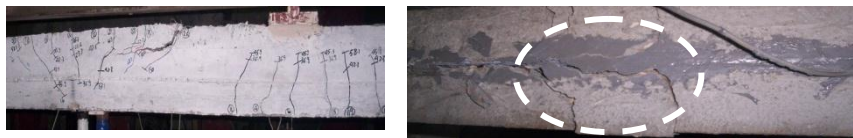
Figure 9. Epoxy split failure: Crack pattern at failure for B3 and B4
