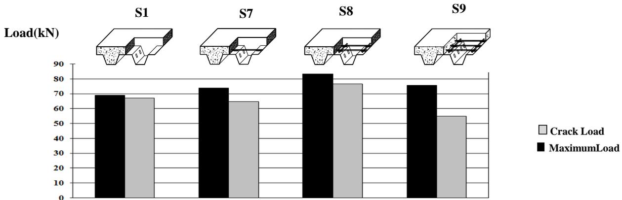
Fig.15: Comparison between Maximum Load and Crack Load for S1, S7, S8, S9
