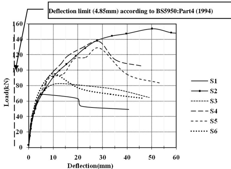
Fig.11: Load –Deflection Curve for Specimens S1 to S6
