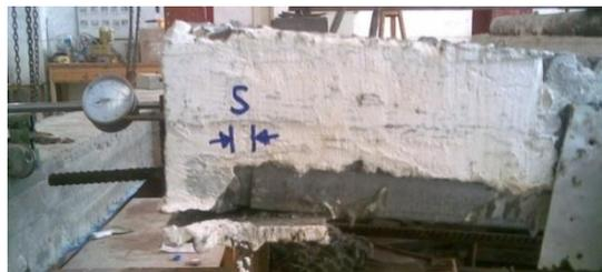
**Fig.12: Slip at left side of specimen s6**
