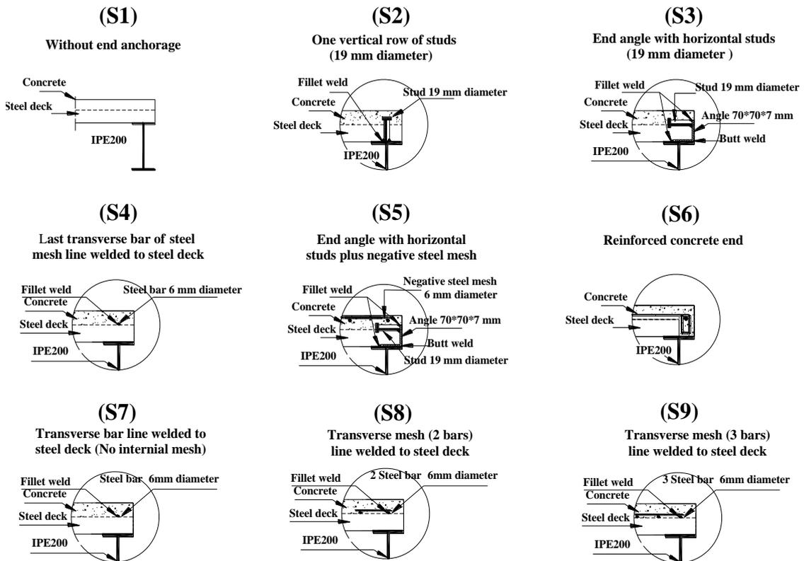
Fig. 8: End Anchorages Details
