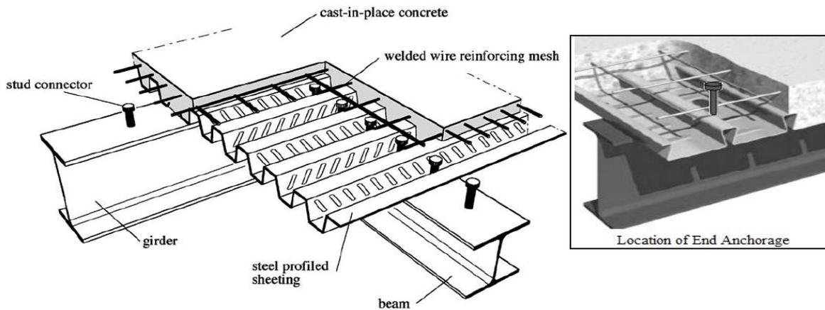
**Fig.1: Composite Floor with Steel Deck**
