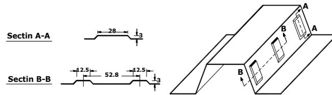
**Fig. 5:Details of Steel Deck Embossments in mm**
