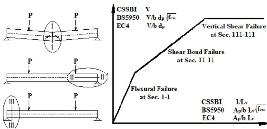
**Fig. 2: Modes of Failure**
