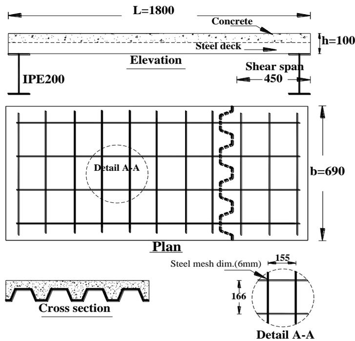
**Fig. 4:Geometry and Basic Dimensions of Specimens in mm**
