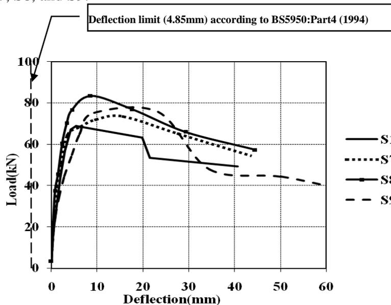
Fig.16: Load –Deflection Curve for Specimens S1, S7, S8, S9
