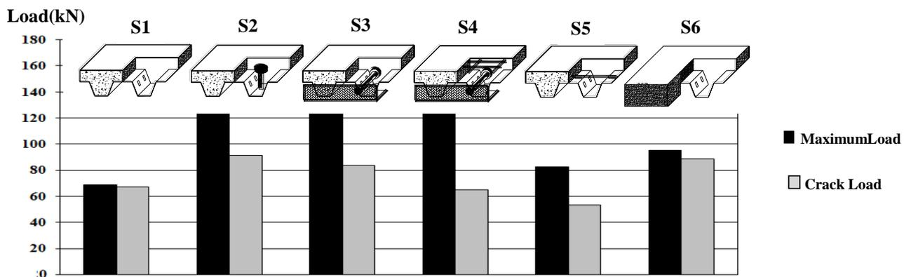
**Fig. 10: Comparison between Maximum Load and Crack Load for S1 to S6**
