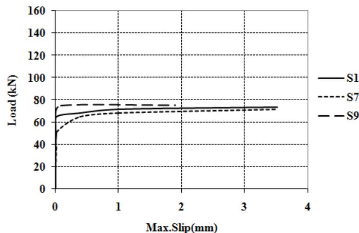
Fig.17: Load –Max. Slip Curve for Specimens S1, S7, S8, S9
