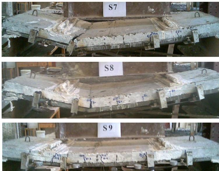
**Fig.14:Cracks Pattern of Composite Slabs without Internal Reinforcement Mesh**
