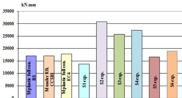
Fig.18: Moment Capacity Comparison for specimens S1to S6
