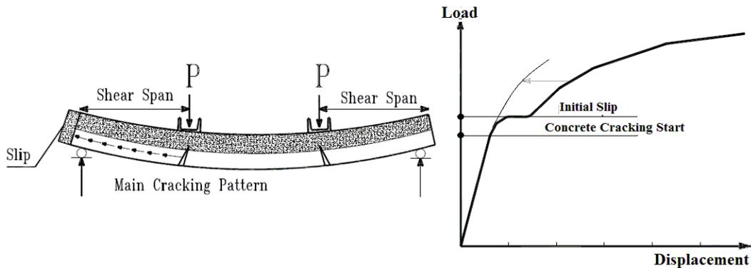
**Fig. 3:Shear Bond Failure**
