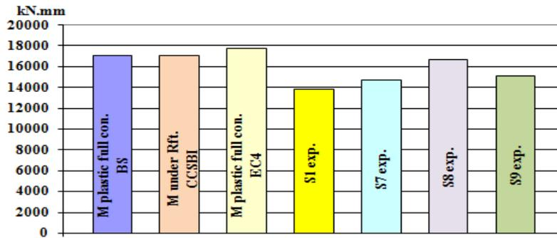
**Fig.19: Moment Capacity Comparison for Specimens S1, S7, S8, S9**
