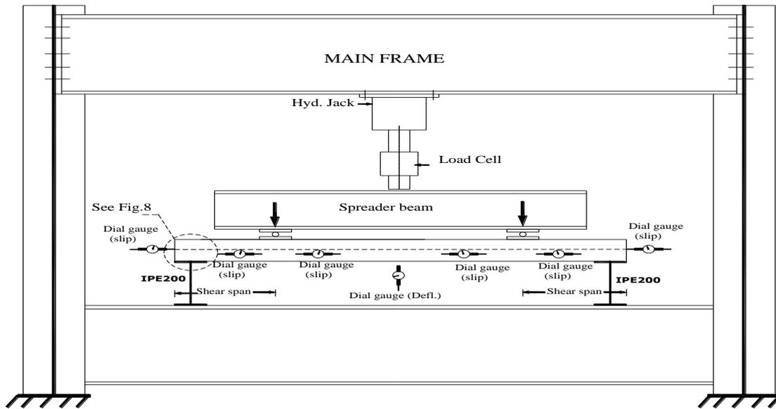
**Fig. 6: Schematic Drawing of Test Set Up**
