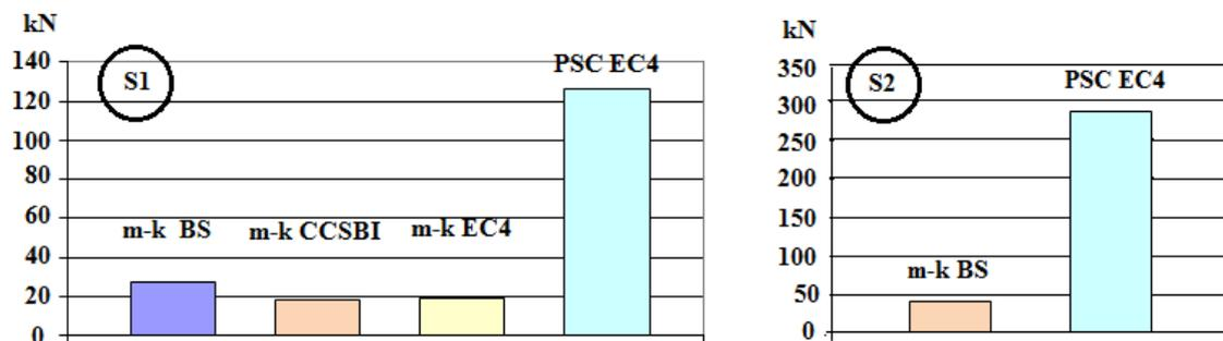
**Fig.20: Shear Bond Capacity for Specimen S1, S2 according to Different Codes**
