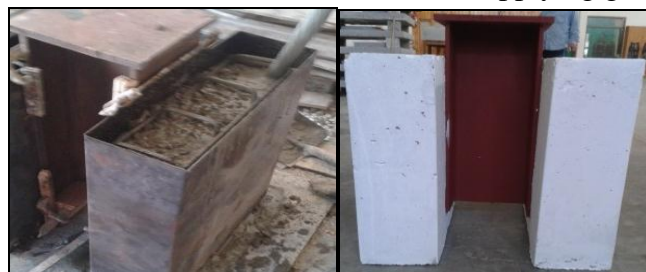
(e) Concrete pouring and (f) Finishing the specimen
