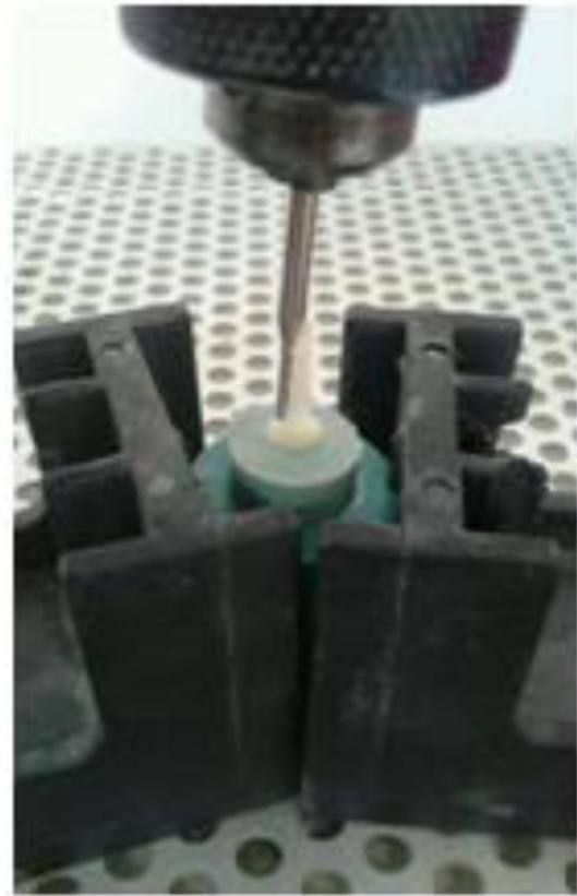
Fig. 1. Milling half of premolar root to generate biological dentine posts.
