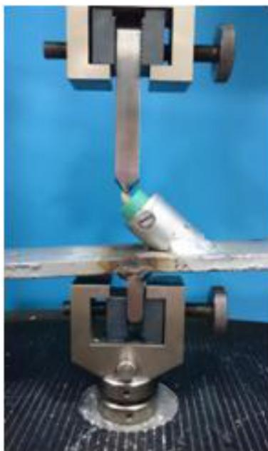
Fig. 4. Fracture resistance testing.
