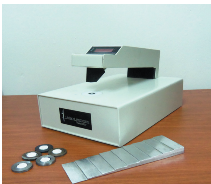
Fig. 1: Densitometer, some specimens and aluminum step wedge used for radiopacity test.
