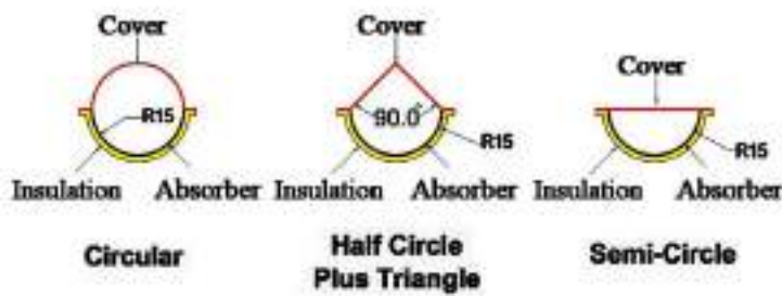
Fig .7. The different three cross section area of tested solar air heater for verification. [19]
