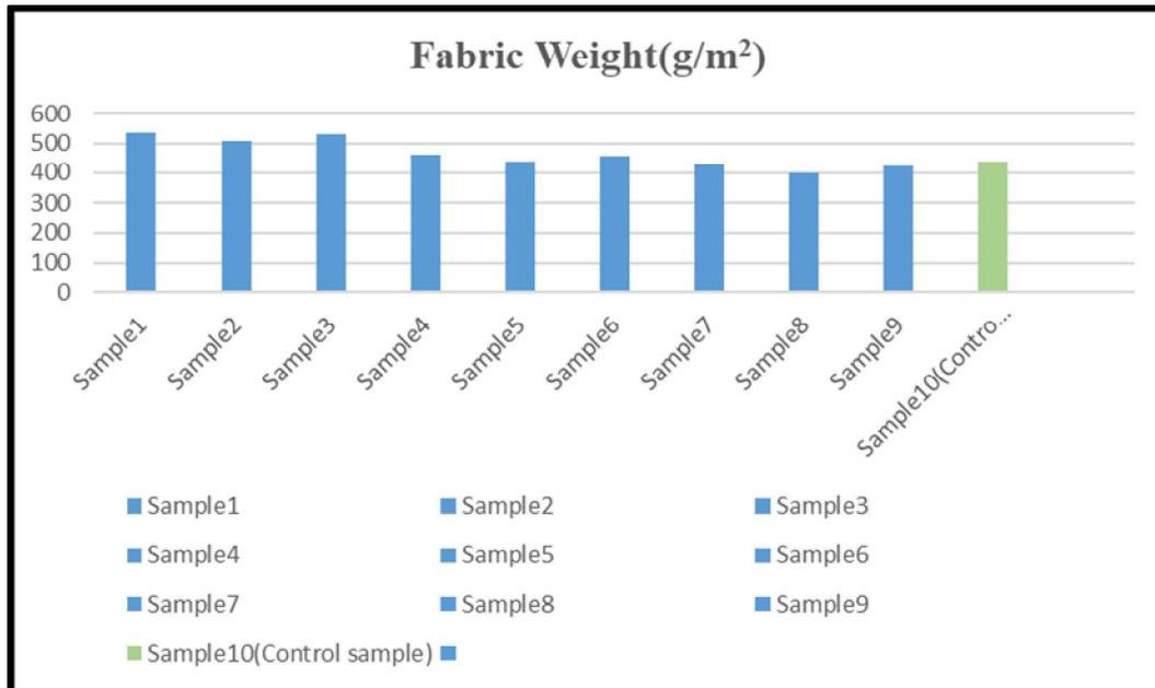
Figure (3) Results of the fabric weight test for the executed samples (g/m<sup>2</sup>)
