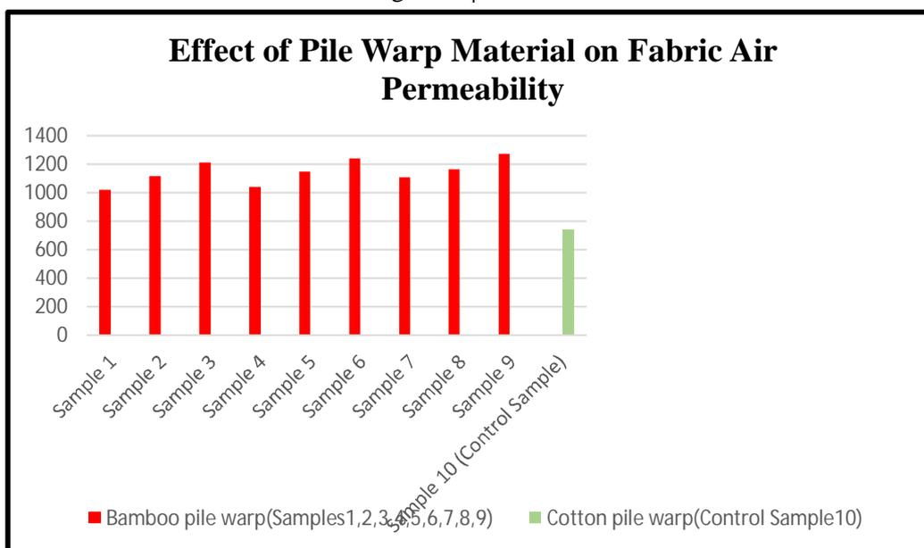
Figure (21) Effect of pile warp material on fabric air permeability (L/m<sup>2</sup>/Sec) for the executed samples.
