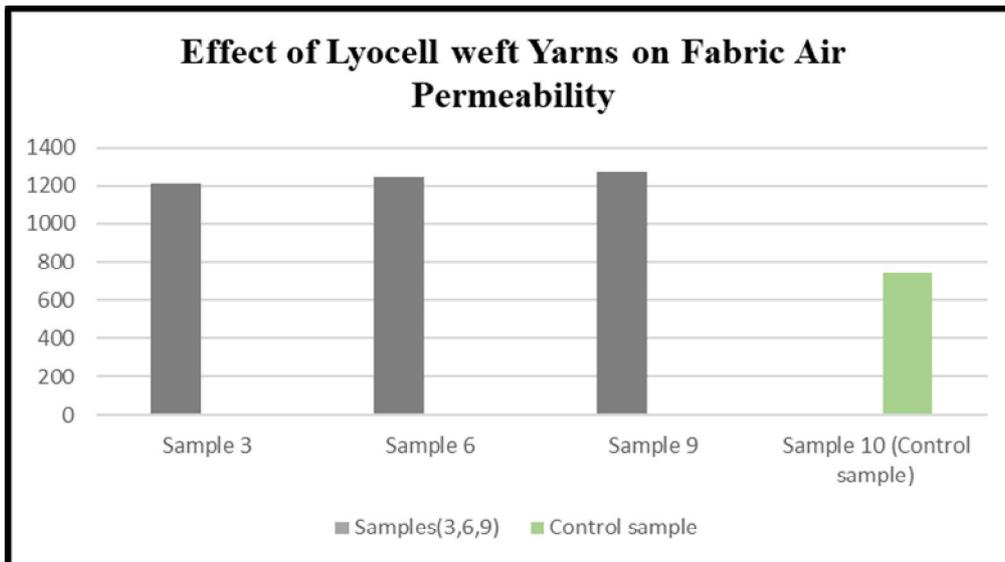
Figure (20) Effect of Lyocel weft material on fabric air permeability (L/m<sup>2</sup>/Sec) for the executed samples
