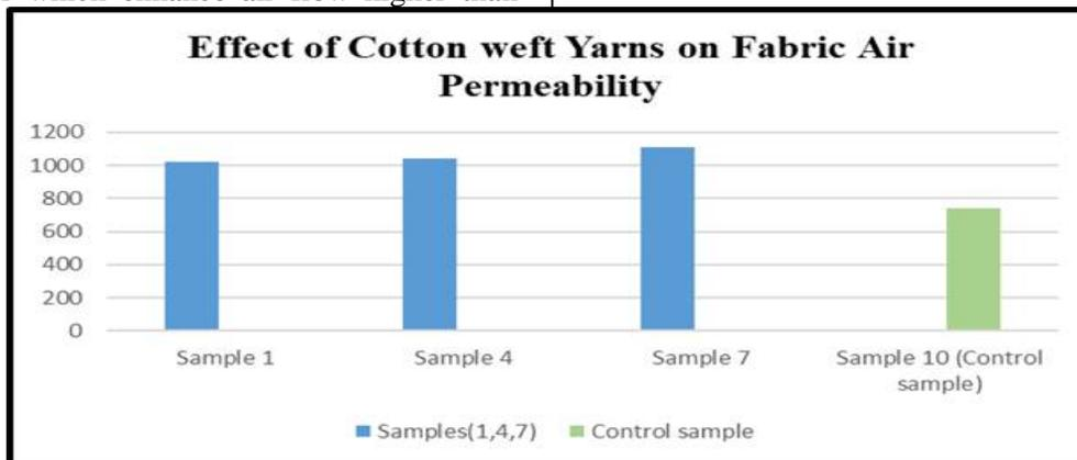
Figure (18) Effect of Cotton weft material on fabric air permeability (L/m<sup>2</sup>/Sec) for the executed samples
