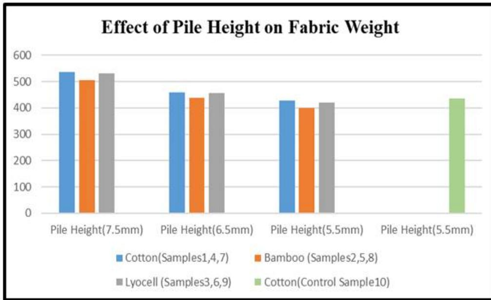
Figure (4) Effect of pile height (mm) on fabric weight(g/m<sup>2</sup>) for the executed samples
