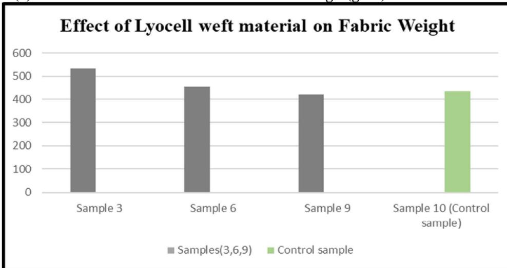
Figure (7) Effect of Lyocell weft material on fabric weight(g/m<sup>2</sup>) for the executed samples
