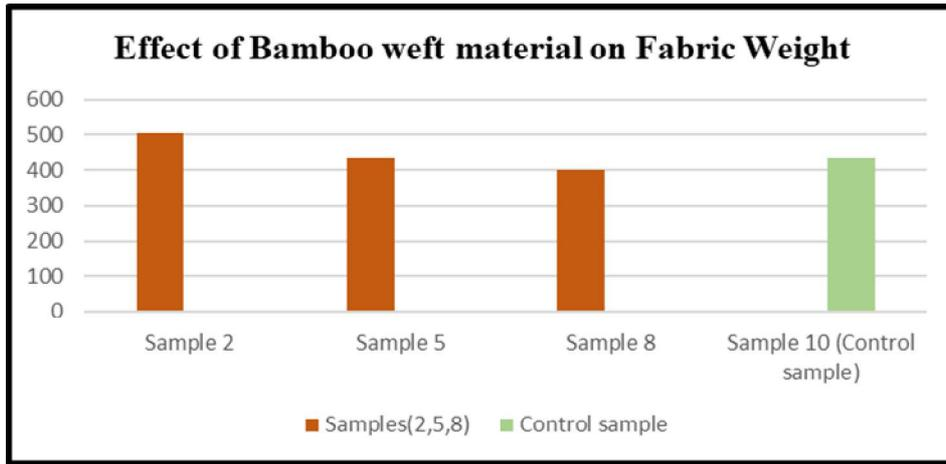
Figure (6) Effect of Bamboo weft material on fabric weight(g/m<sup>2</sup>) for the executed samples
