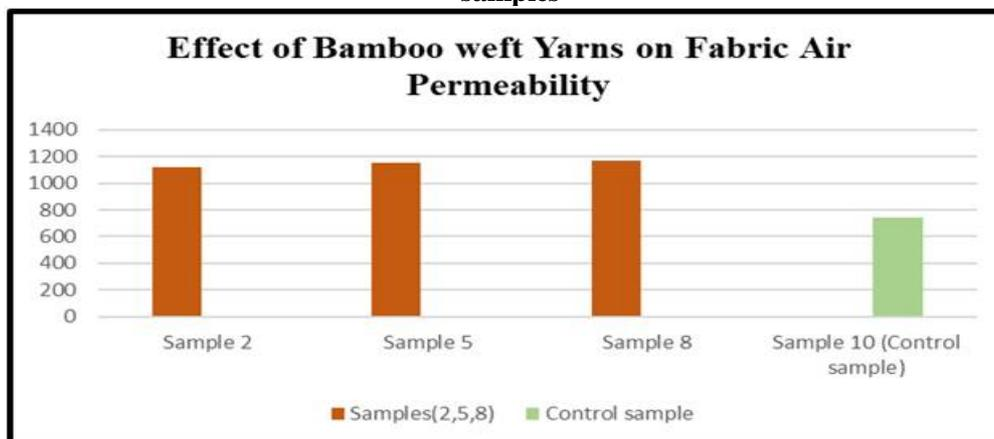
Figure (19) Effect of Bamboo weft material on fabric air permeability (L/m<sup>2</sup>/Sec) for the executed samples
