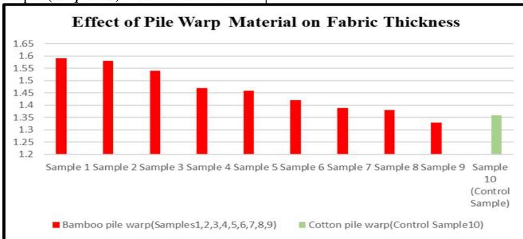
**Figure (14) Effect of pile warp material on fabric thickness (Cm) for the executed samples**
