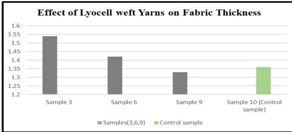
**Figure (13) Effect of Lyocell weft material on fabric thickness (Cm) for the executed samples**
