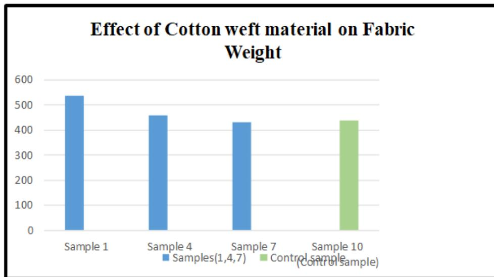
Figure (5) Effect of Cotton weft material on fabric weight(g/m<sup>2</sup>) for the executed samples
