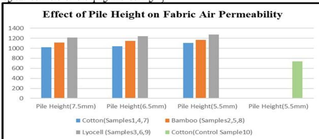
**Figure (16) Effect of pile height (mm) on fabric air permeability (L/m²/Sec) for the executed samples**
