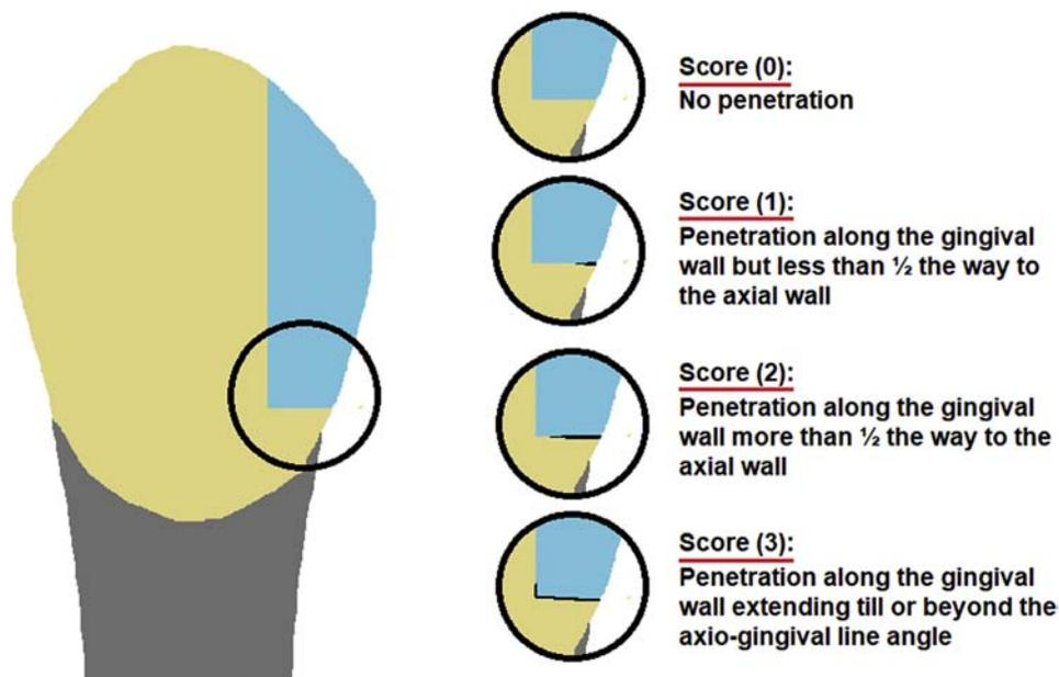
Fig. 2. Schematic representation of the criteria used for microleakage scoring.
