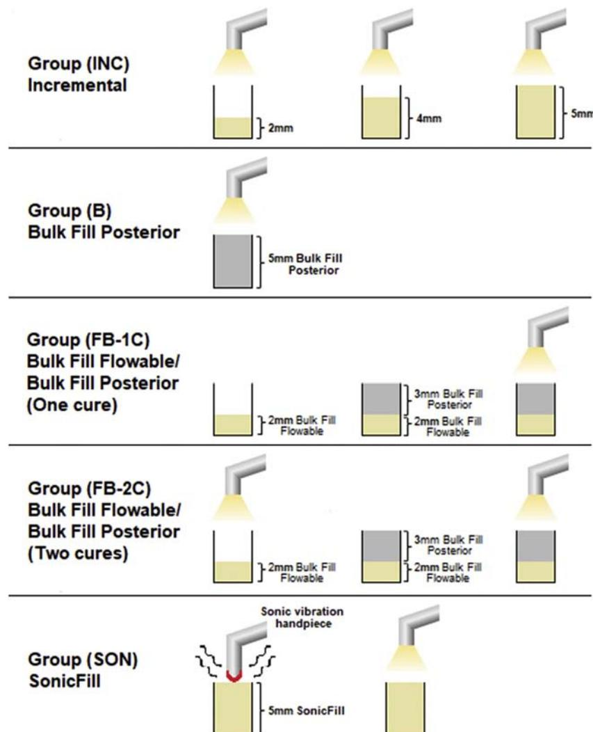
Fig. 1. Schematic illustration of the different material/restorative technique combinations.
