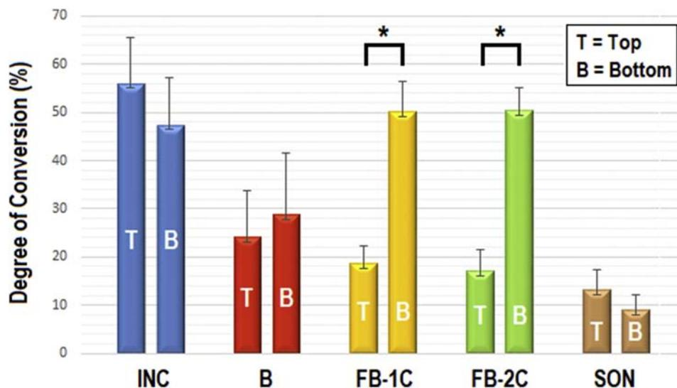
Fig. 4. Comparison between the DC of the top and bottom surfaces of each single group.
