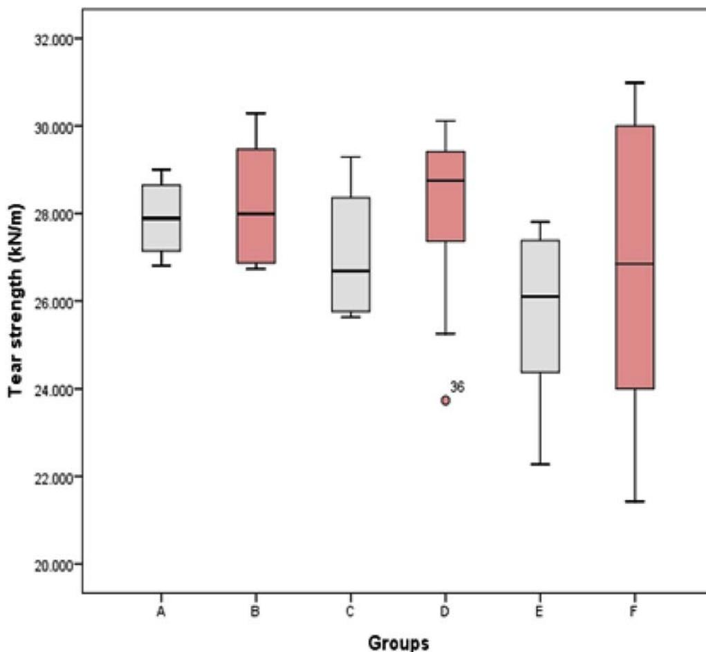
Fig. 3. Box plot presentation of tear strength mean value of all study groups in kN/m.
