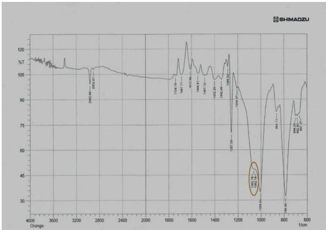
Fig. 7. FTIR spectrum for pigmented sample.
