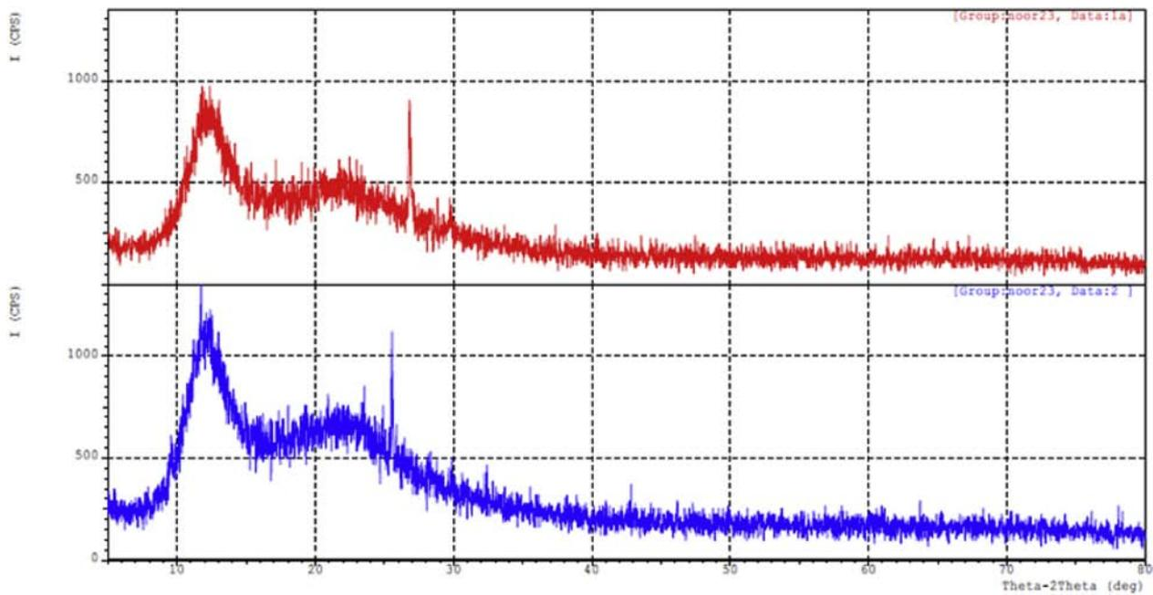
Fig. 8. XRD patterns for the non-pigmented sample (red peaks) and the pigmented sample (blue peaks).
