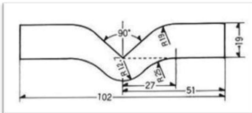
Fig. 2. Type C tear strength test sample dimensions in mm (adopted from ASTM D624, 2013).
