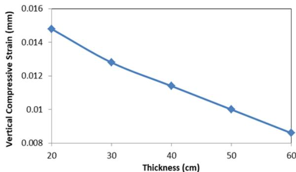
Figure 3. Relationship between the thickness of base course layer and vertical compressive strain at the top of subgrade layer (9% lime)
