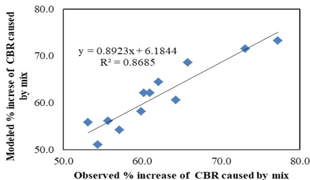
Figure 2. Modeled and measured increase percentages of CBR for lime - sodium chloride mix
