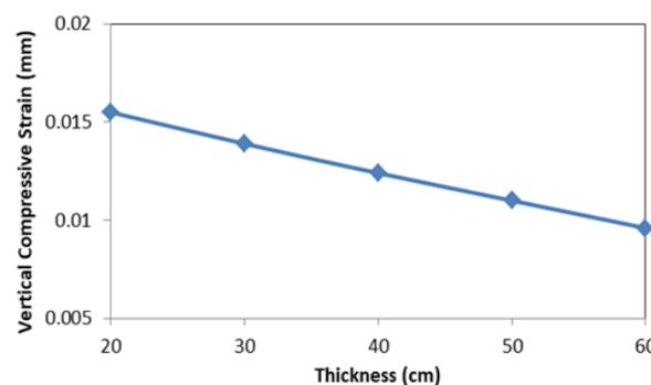
Figure 4. Relationship between the thickness of base course layer and vertical compressive strain at the top of subgrade layer (5% sodium chloride)
