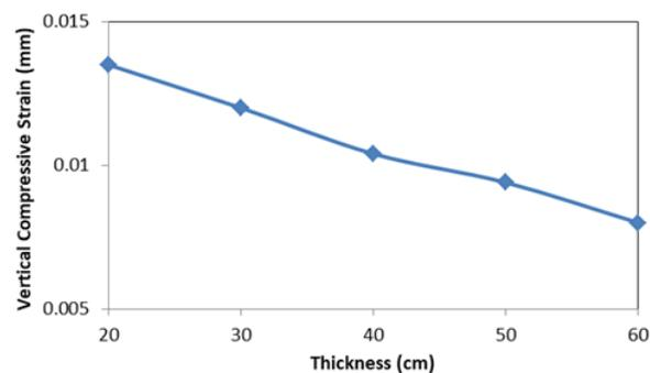
Figure 5. Relationship between the thickness of base course layer and vertical compressive strain at the top of subgrade layer (10% organic polymer)
