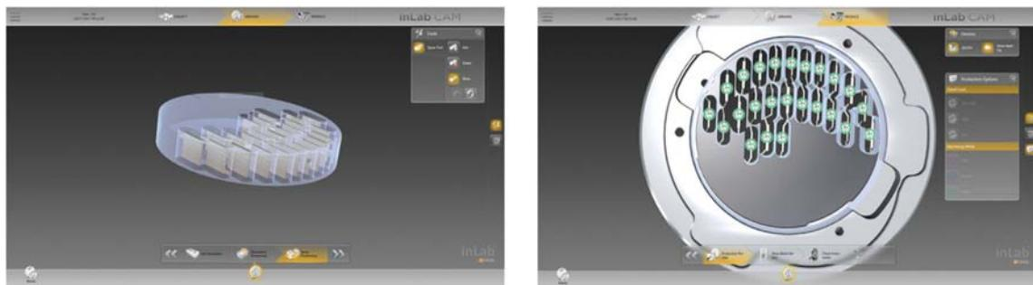
Fig. 1. Software design for zirconia specimens before milling.
