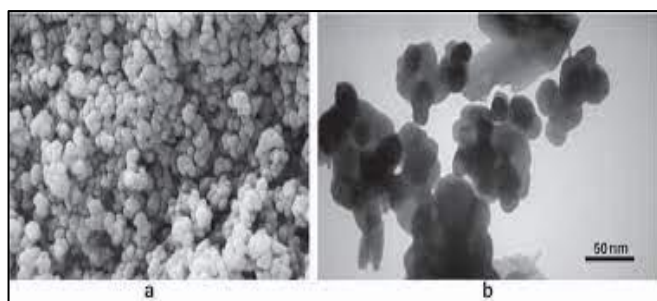
Figure 1: Copper oxide TEM micrograph (Adapted from [99])
