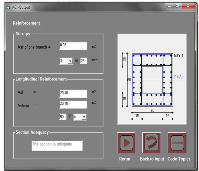
Figure 4. Output data for box section
