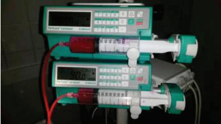
Fig. 1: The two electric push-syringes with the contrast solution inside the 60 ml syringes.
