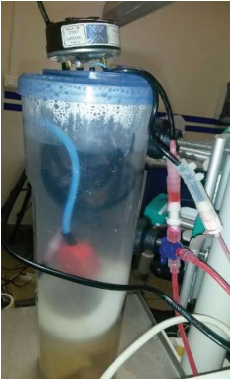
Fig. 3: The T-connector that connects the two syringes to the 3m tube in order to heat the solution to 60 °C.
