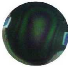
Figure 1: Photograph of 3C-SiC thin film deposited on thermally oxidized Si
