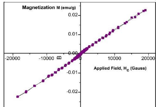
Figure 7: VSM loop of the ZnO nanoparticles
