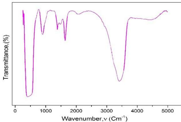
Figure 6: FTIR spectrum of the ZnO nanoparticles.
