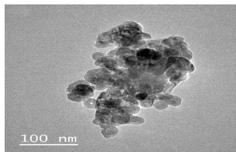
Figure 4: TEM image of the prepared ZnO nanoparticles.
