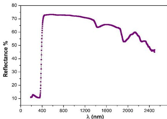
Figure 8: The DRS of the ZnO nanoparticles.
