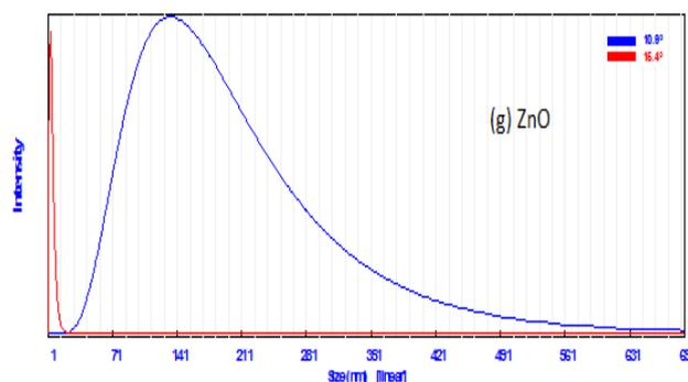
Figure 3: the PSD of the ZnO nanoparticles.
