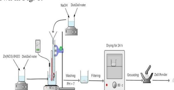
Figure 1: The preparation steps of ZnO nanoparticles.
