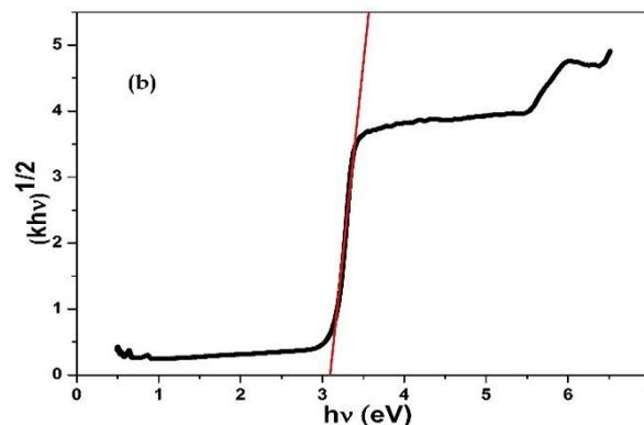
Figure 9: (a) direct bandgap and (b) the indirect band gap Taucs plot.
