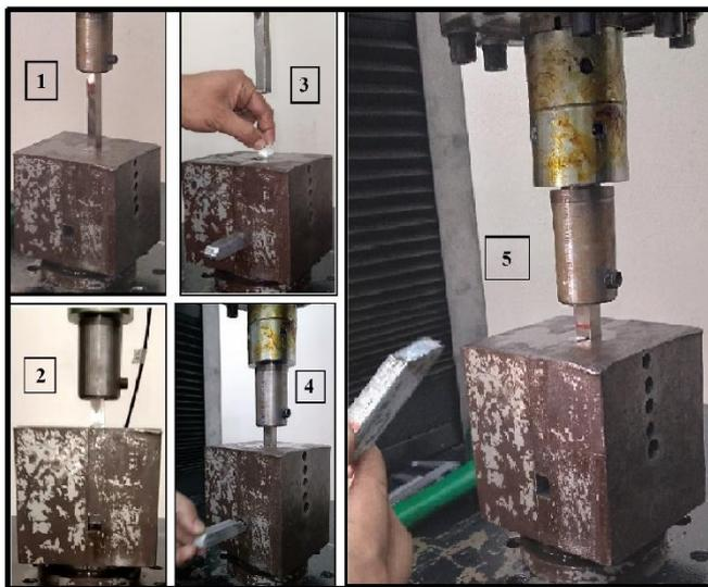
Fig. 4 The billet during ECAP
