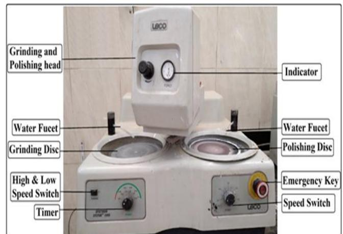
Fig. 7. Spectrum System 1000 (SS-1000) Grinder/Polisher machine
