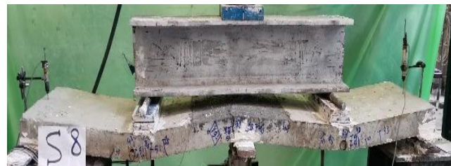
(h) Crack pattern of specimen S_8
