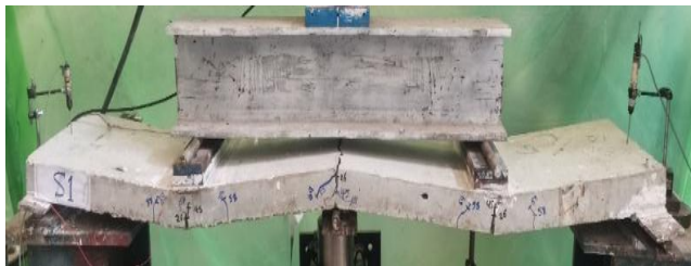
(a) Crack pattern of specimen S_1
