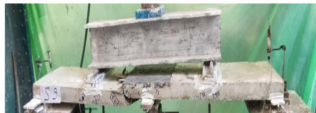
(j) Crack pattern of specimen S_9
