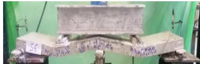
(f) Crack pattern of specimen S_6
