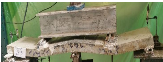
(c) Crack pattern of specimen S_3
