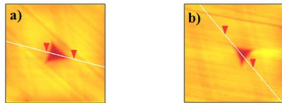
**Figure 3:** Atomic force microscopic images of indentations created in the surfaces of samples: (a) Sample c<sub>2</sub> and (b) sample c<sub>5</sub>.
