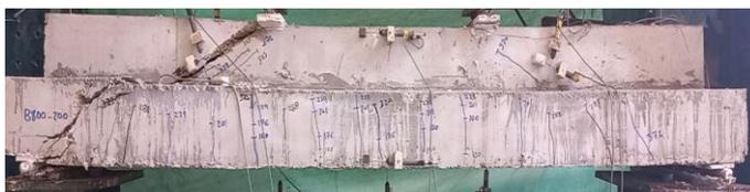
(e) Crack patterns of B<sub>5</sub>
