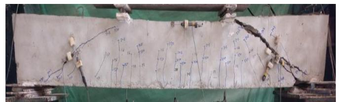
**(a) Crack patterns of  $B_0$**
