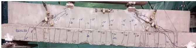
(b) Crack patterns of B<sub>2</sub>
