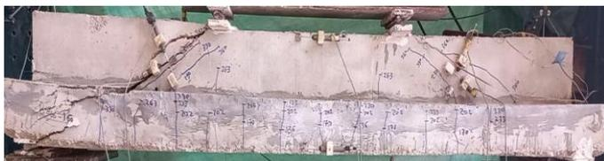
(c) Crack patterns of B<sub>3</sub>
