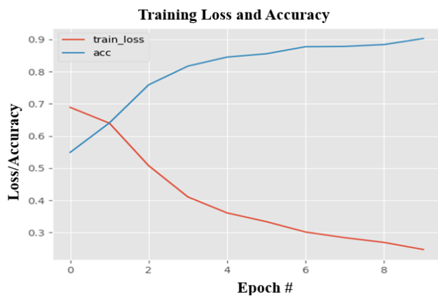
Figure 10. Training loss and accuracy of our CNN- smile detection with 10 epochs on GENKI-4k dataset
