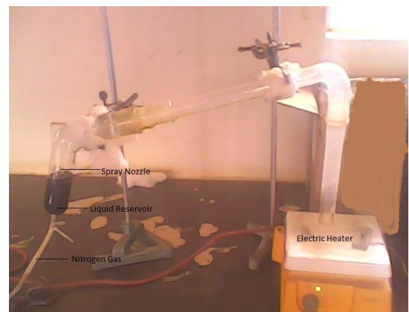
Figure 2: A photograph of set up that was used in the film deposition.
