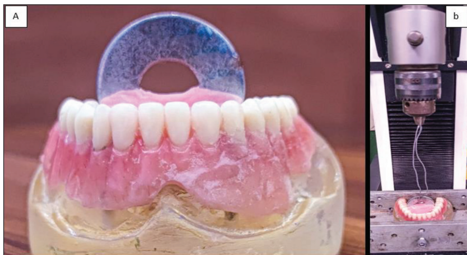
Figure (5) A: Denture With Cylinder Attached To Geometric Centre. B: Insertion And Removal Cycles At Universal Testing Machine
