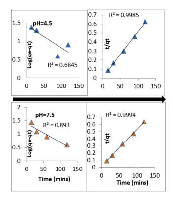
**Figure 9.** The kinetic models, for  $Pb^{2+}$  removal and efficiency of contact time by *Sargassum* sp in pH value 4.5 and 7.5 at 20B station in summer season.
