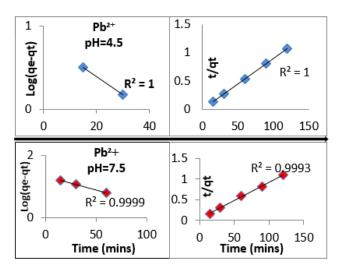
**Figure 7.** The kinetic models for Pb<sup>2+</sup> removal and efficiency of contact time by *Sargassum* sp in pH value 4.5 and 7.5 at 20B station in winter season
