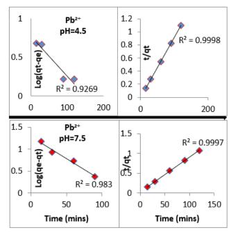
**Figure 6.** Kinetic models for  $Pb^{2+}$  removal and efficiency of contact time by *Gracilaria* sp in pH value 4.5 and 7.5 at 20B station in winter season.
