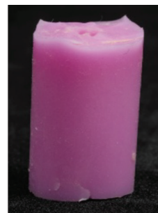
Figure (5) — Silicone impression of male part
