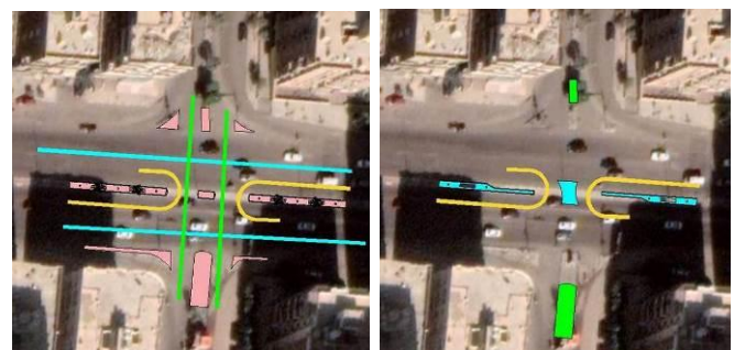
Figure 30. The two proposed solutions by the research; a) on the left is reopening a four-way intersection and b) on the right is opening just a U-turn [16] (Edited by the Author)
