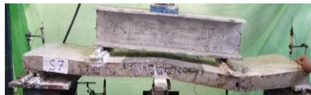
(g) Crack pattern of specimen S_7
