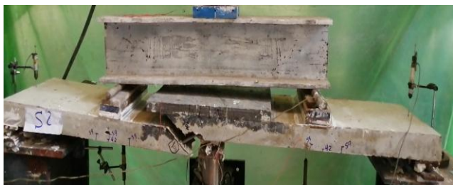
(b) Crack pattern of specimen S_2
