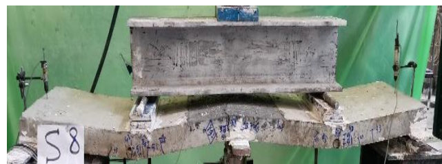
(h) Crack pattern of specimen S_8
