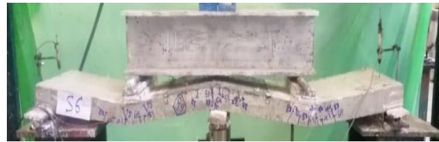
(f) Crack pattern of specimen S_6
