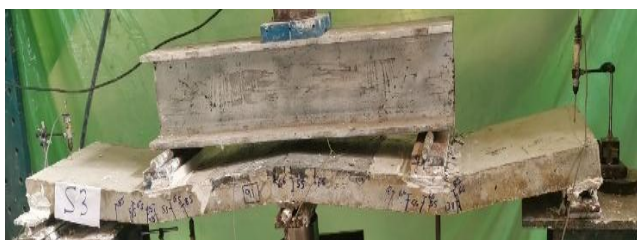
(c) Crack pattern of specimen S_3
