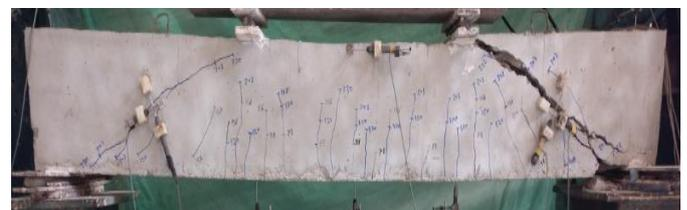
**(a) Crack patterns of  $B_0$**
