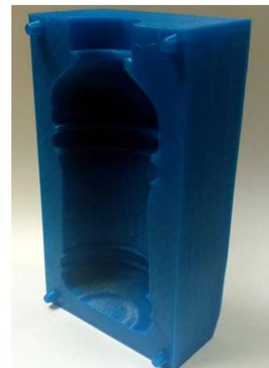
**Figure 10: Printed blowing mold**
