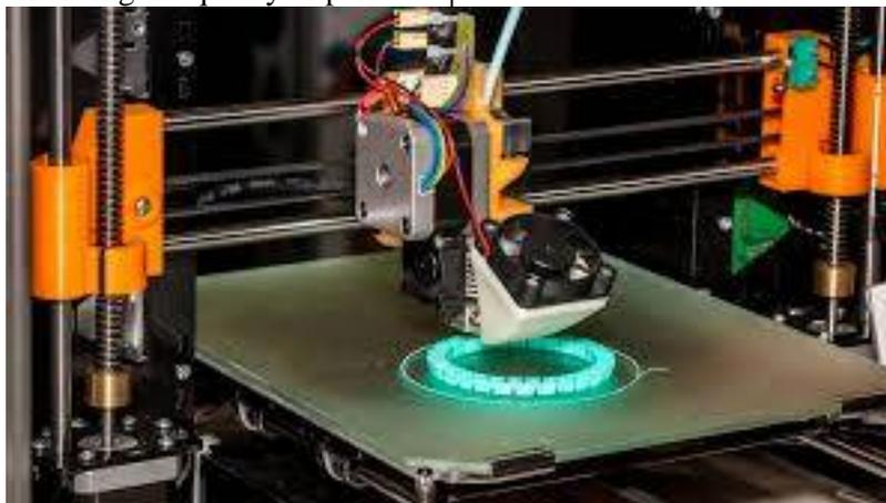
**Figure 4:** Fused Deposition Modeling 3d printer
