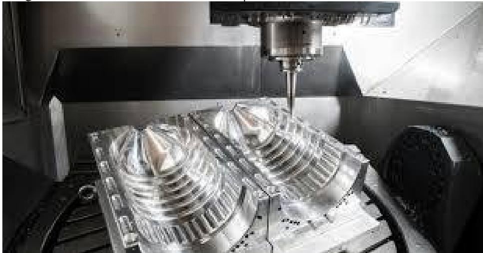
**Figure 3:** CNC milling metal blowing mold
