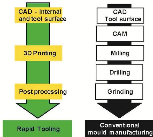
**Figure 2:** Conventional mold manufacturing and rapid tooling
