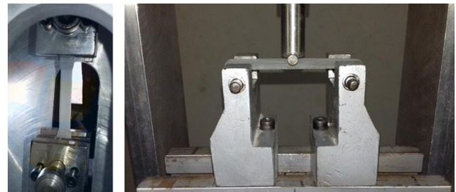
b) Tensile and flexure testing setup for fabric and polyester specimens.
