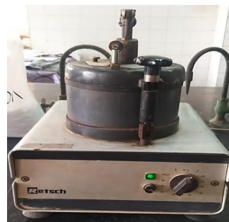
Fig. 3: Grinder used for crushing seashell and eggshell.
