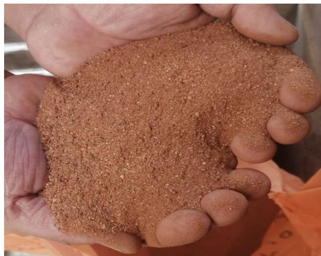
Figure 3. Grinded broken bricks in its natural form [Source: author]
