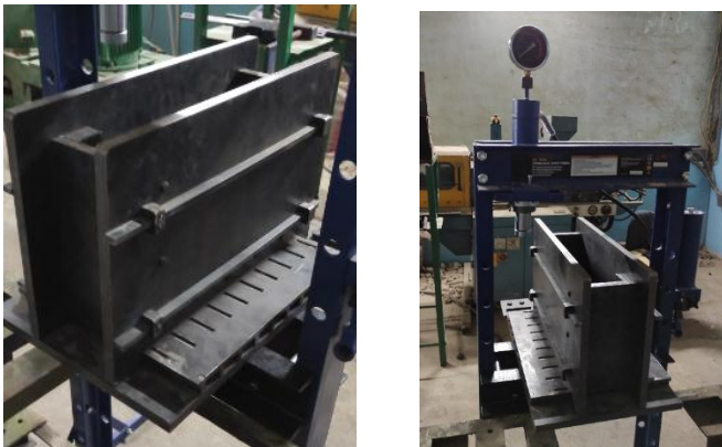
Figure 6. Brick mold, and Hydraulic piston [Source: author]
