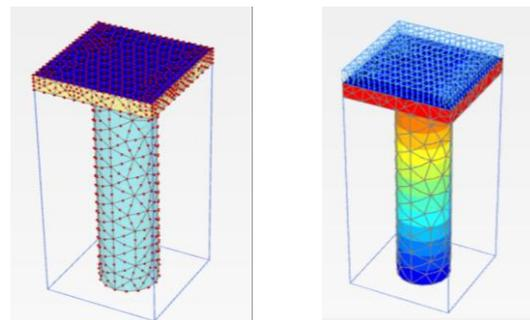
Figure 6-a: The mesh generated      Figure 6-b: The deformed mesh
