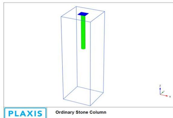
Figure 3. 3D mesh generation ordinary stone column
