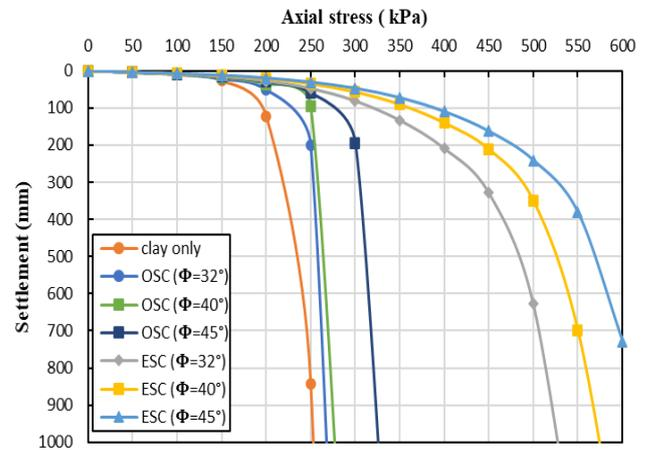
Figure 8. Axial stress – settlement curves for different ( $\phi$ ) (D =0.40 m,  $c_u = 20 \text{ kN/m}^2$ ,  $L_{enc}/D=5$ ,  $J =2000 \text{ kN/m}$ )
