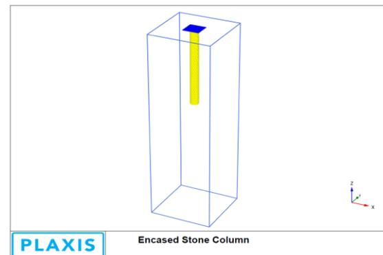
Figure 4. 3D mesh generation fully encased stone column
