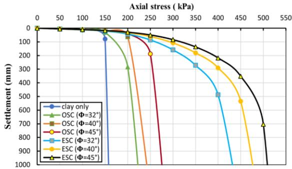
Figure 9. Axial stress – settlement behaviour for different ( $\phi^\circ$ ) ( $D=0.60$  m,  $c_u=20$  kN/m<sup>2</sup>,  $L_{enc}/D=5$ ,  $J=2000$  kN/m)
