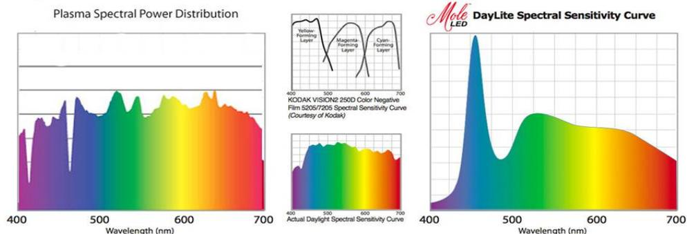
**Figure 8 the spectral power distribution for the Plasma and LED**
