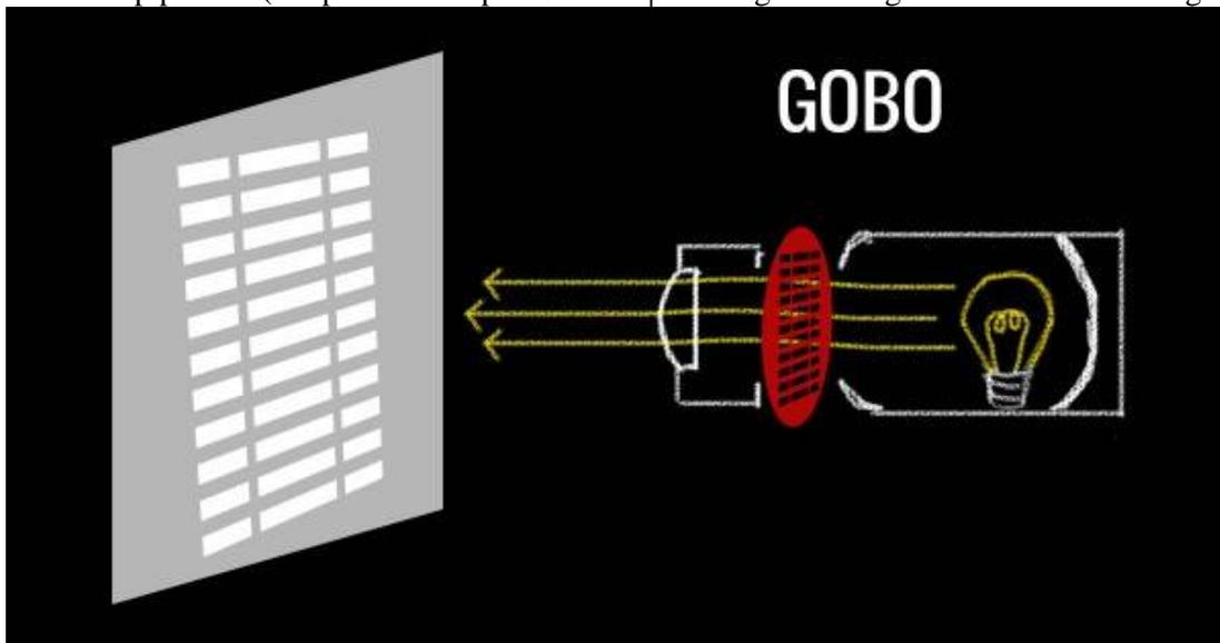
Figure 4 shows gobos drawing a window pattern.
