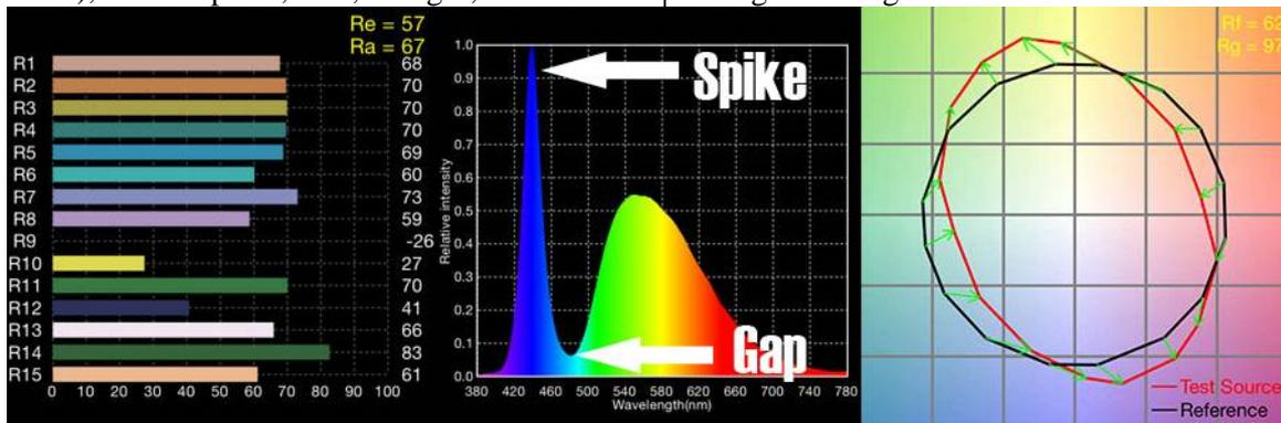
Figure 9 showing the spikes and gaps in The LEDs light color spectrum
