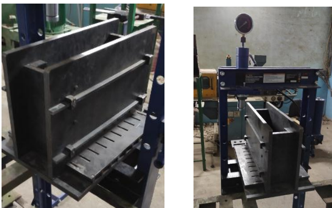
Figure 6. Brick mold, and Hydraulic piston [Source: author]
