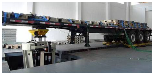
Figure 6 Modal test on the semi-trailer chassis
