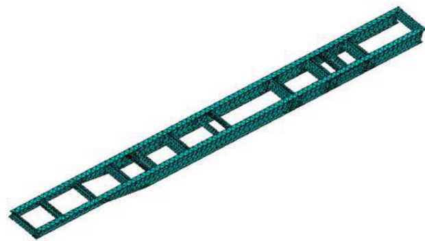
Figure 5 Flexible semi-trailer chassis
