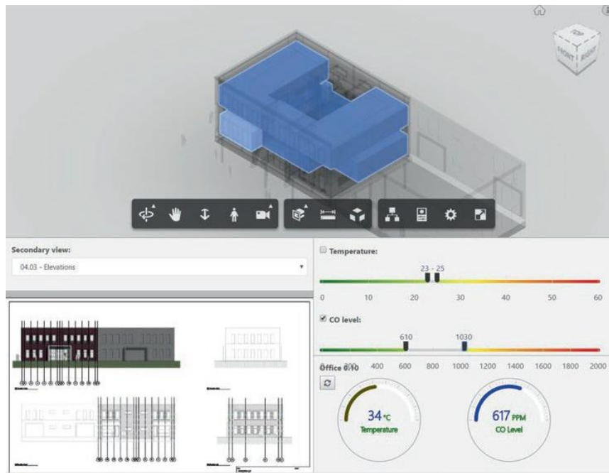
Figure 2. Spatial analysis of room parameters in the BIM model. (Source:[16])
