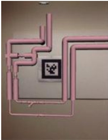
Figure 16. Virtual piping system behind the wall.
