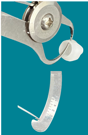
Fig 1. measuring the marginal thickness of one FEFL crown
