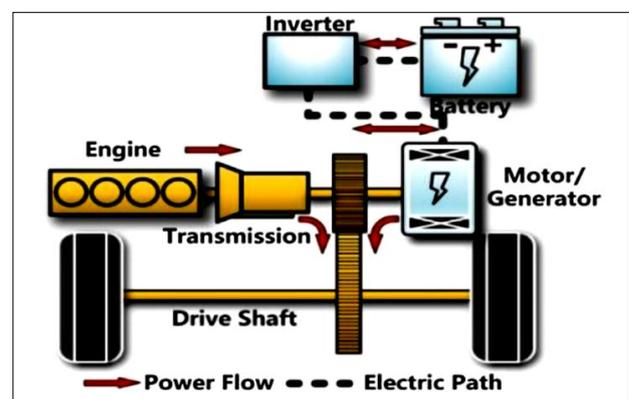
Figure 10. Configuration of parallel HEV [16]
