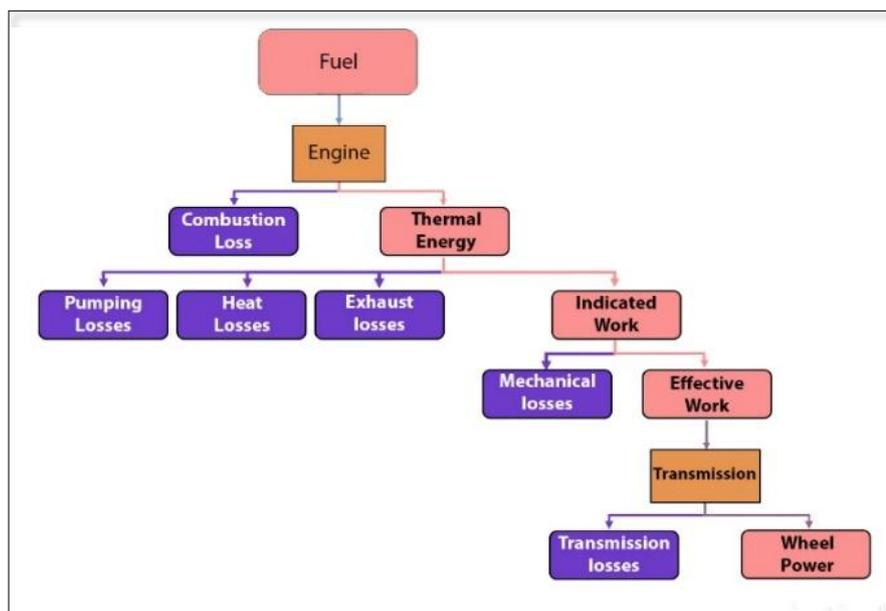
Figure 15. The energy flow distribution and path for conventional vehicles
