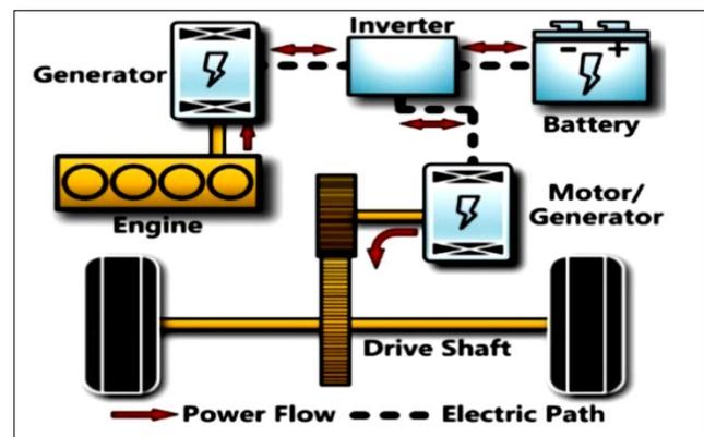
Figure 9. Configuration of series HEV [16].
