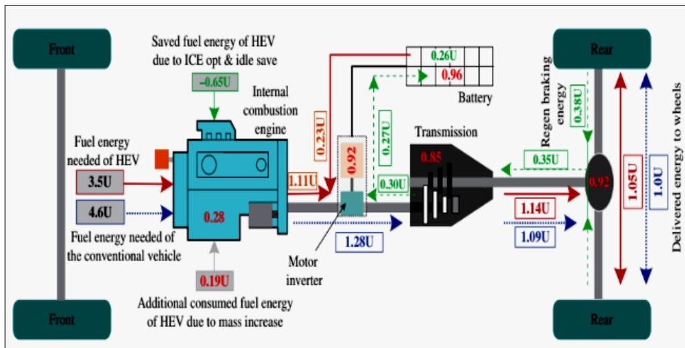
Figure 18. Typical urban cycle energy flows of a conventional powertrain and a hybrid electrified powertrain [19].
