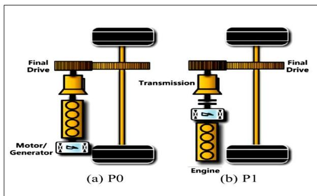
Figure 11. Configurations of subtypes P0, and P1 in parallel HEVs [16]
