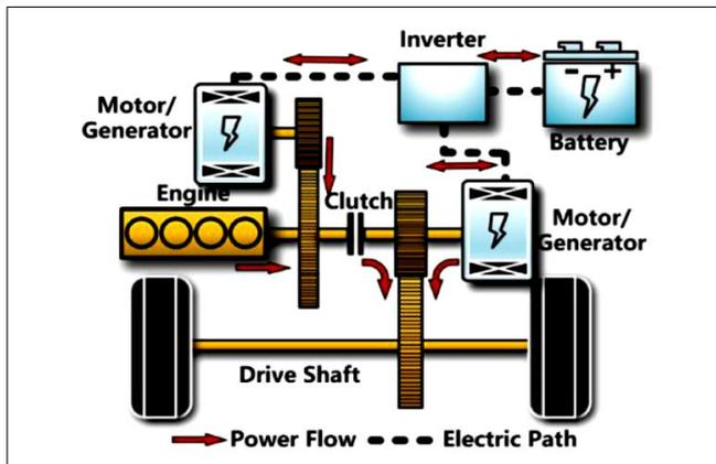
Figure 14. Configuration of series-parallel hybrid powertrain [16]
