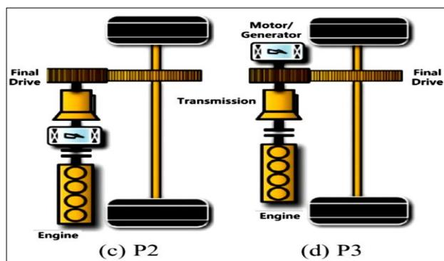
Figure 12. Configurations of subtypes P2 and P3 in parallel HEVs [16]
