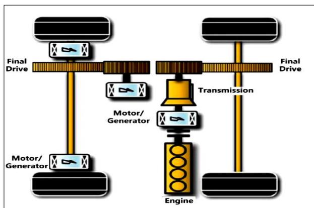
Figure 13. Configurations of subtype P4 in parallel HEVs [16]
