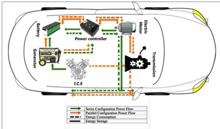
Figure 17. Power flow of a series and parallel hybrid electric vehicle
