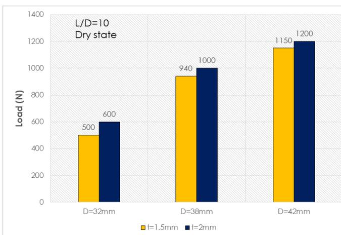
Figure 15. The ultimate pile capacities embedded length (L/d) =10, dry state.
