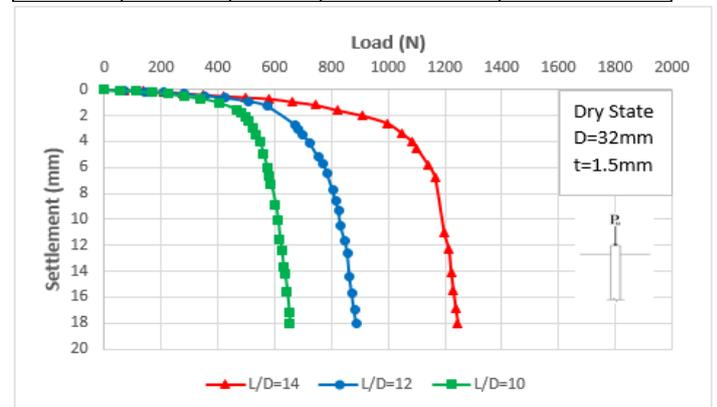
Figure 18. Load-settlement curves for tube piles of different embedded pile lengths, dry state.
