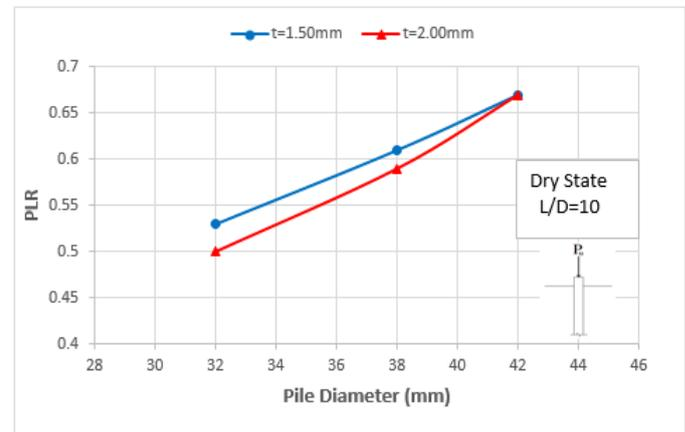
Figure 21. The relation between pile diameter and plug length ratio (PLR) for the dry state, with different pile diameters and different pile thickness.
