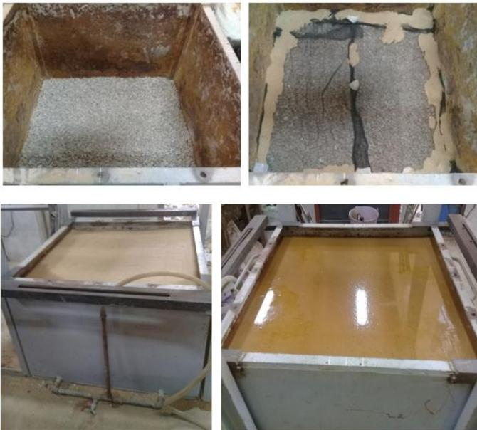
Figure 5. Water was provided from the bottom of the sand bed
