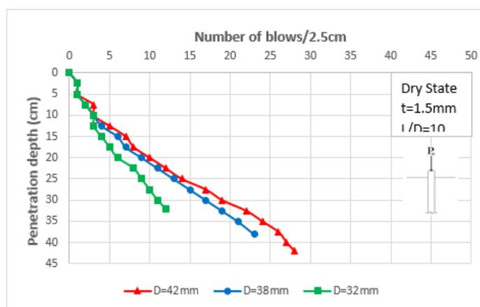
Figure 24. The relation between the number of blows and embedded pile length for different pile diameters at the same pile thickness.
