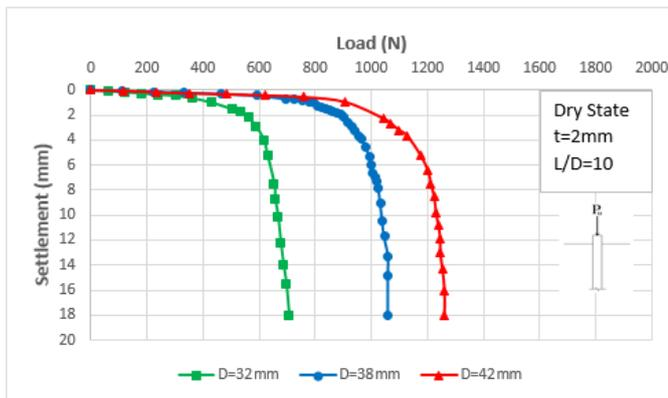
Figure 17. Load-settlement curves for tube piles of 2-mm thickness in a dry state.
