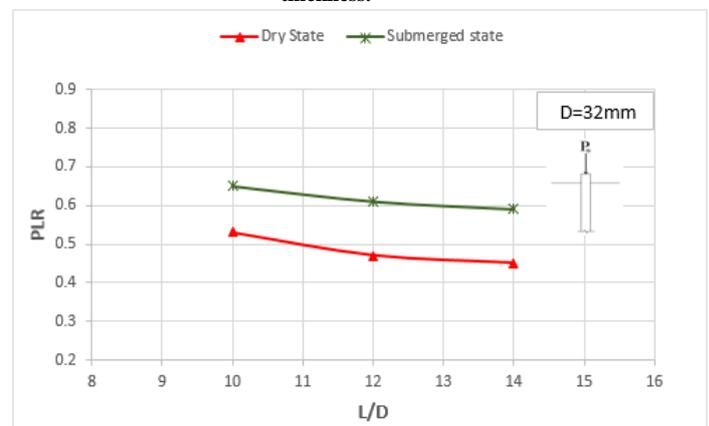
Figure 22. The relation between embedded pile length and plug length ratio (PLR) for dry and submerged states
