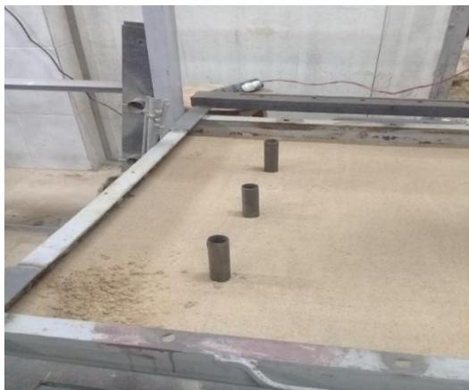
Figure 8. Steel pipe-pile after installation
