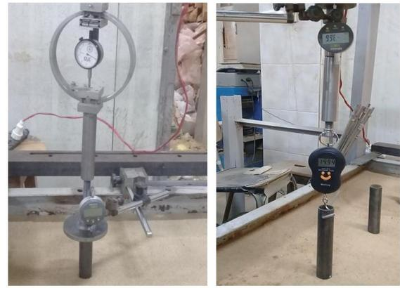
Figure 4. Proving ring with dial gauge 0.002 mm accuracy and a Sensitive balance.
