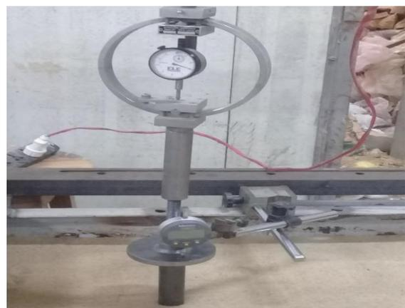
Figure 9. Pile loading for the test (1) and test (2).
