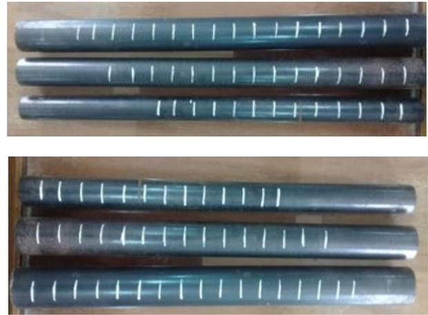
Figure 1. Models of steely tube piles with two different pile thicknesses of (1.5 and 2) mm and pile diameters (32, 38, and 42) mm.
