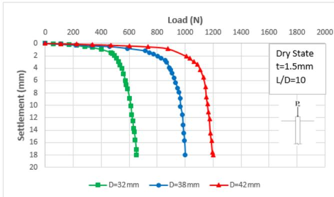
Figure 16. Load-settlement curves for tube piles of 1.5-mm thickness in a dry state.
