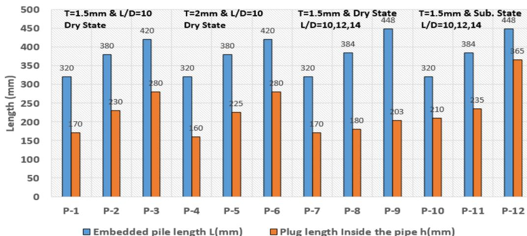
Figure 23. The relation between embedded pile length and plug length inside the pipe
