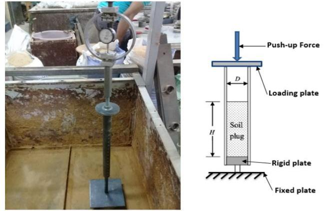
Figure 12. Push-up loading to determine the internal friction for the tube pile.
