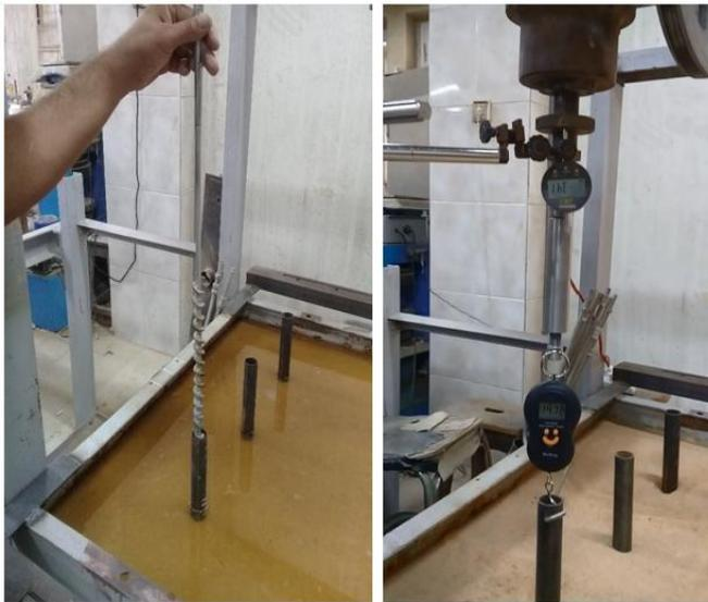
Figure 11. Pile loading for the test (3) and Soil plug removal tool.
