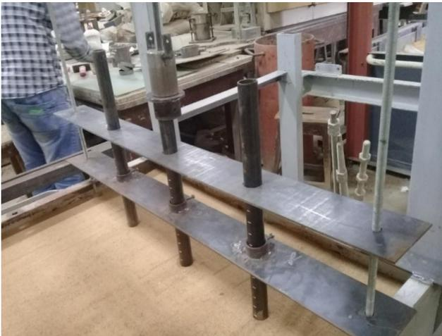
Figure 7. Driven the pile models.
